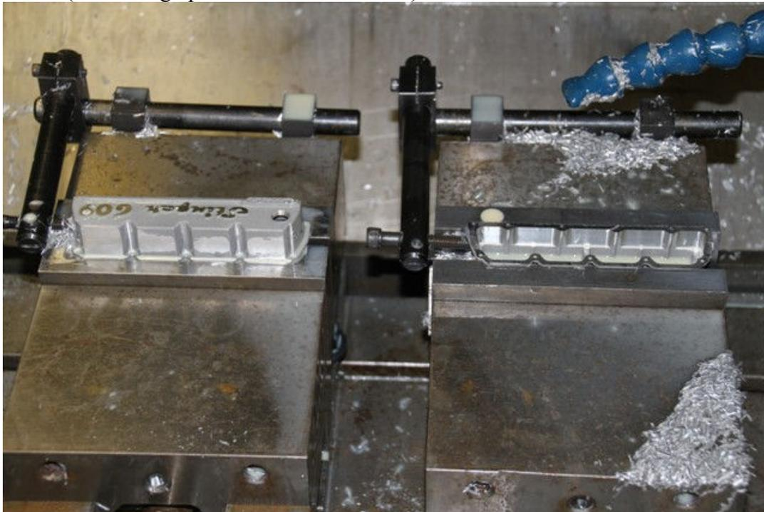
Pic #4 (Three stages of completion on valve covers)
