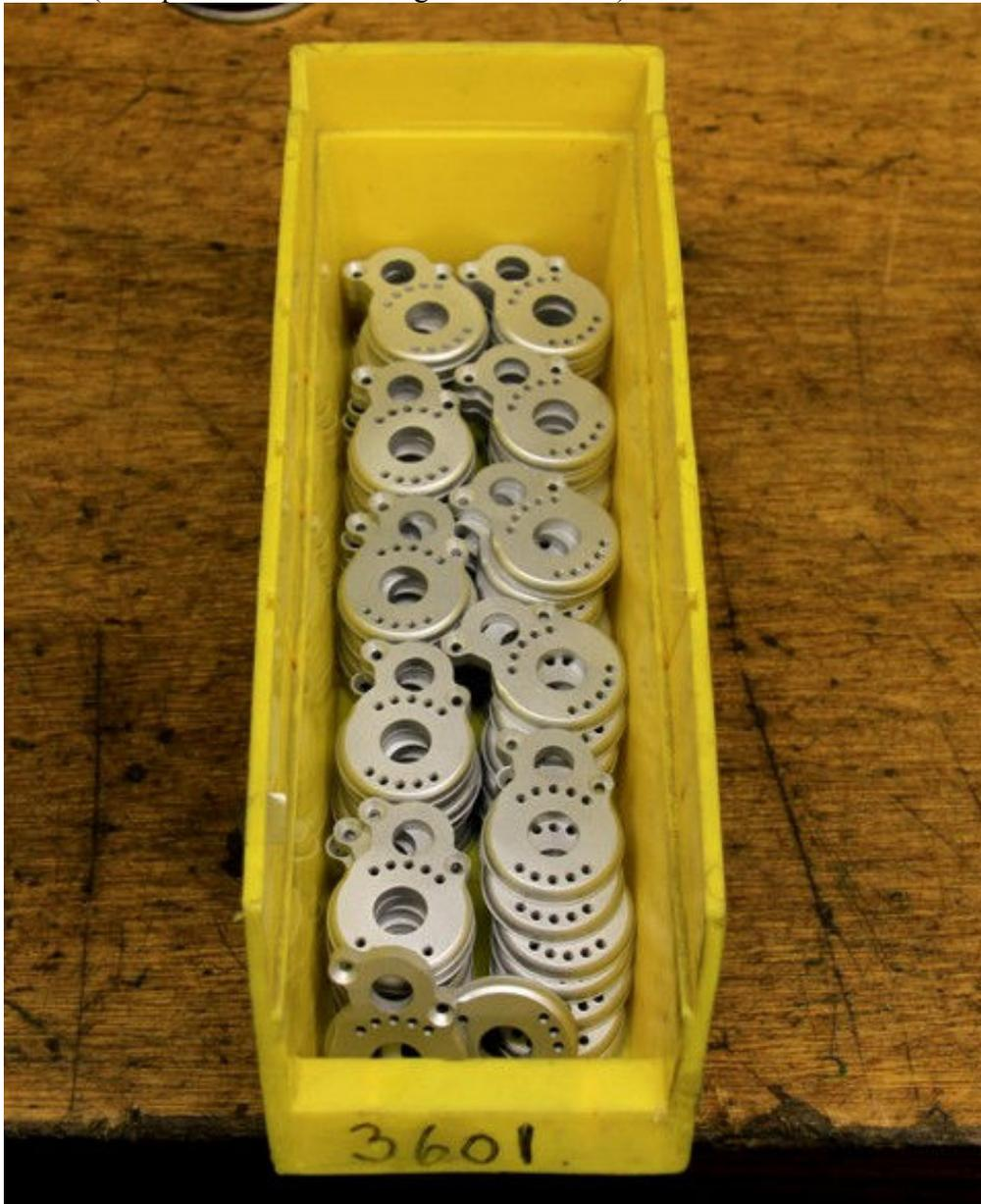
Pic #8 (Second half of starter motor gear case)
