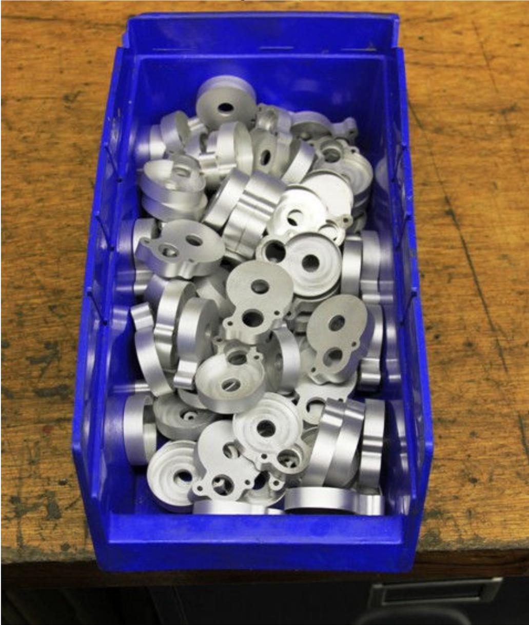
Pic #9 & 10 (Machining bearing support for new starter motor gear case)
