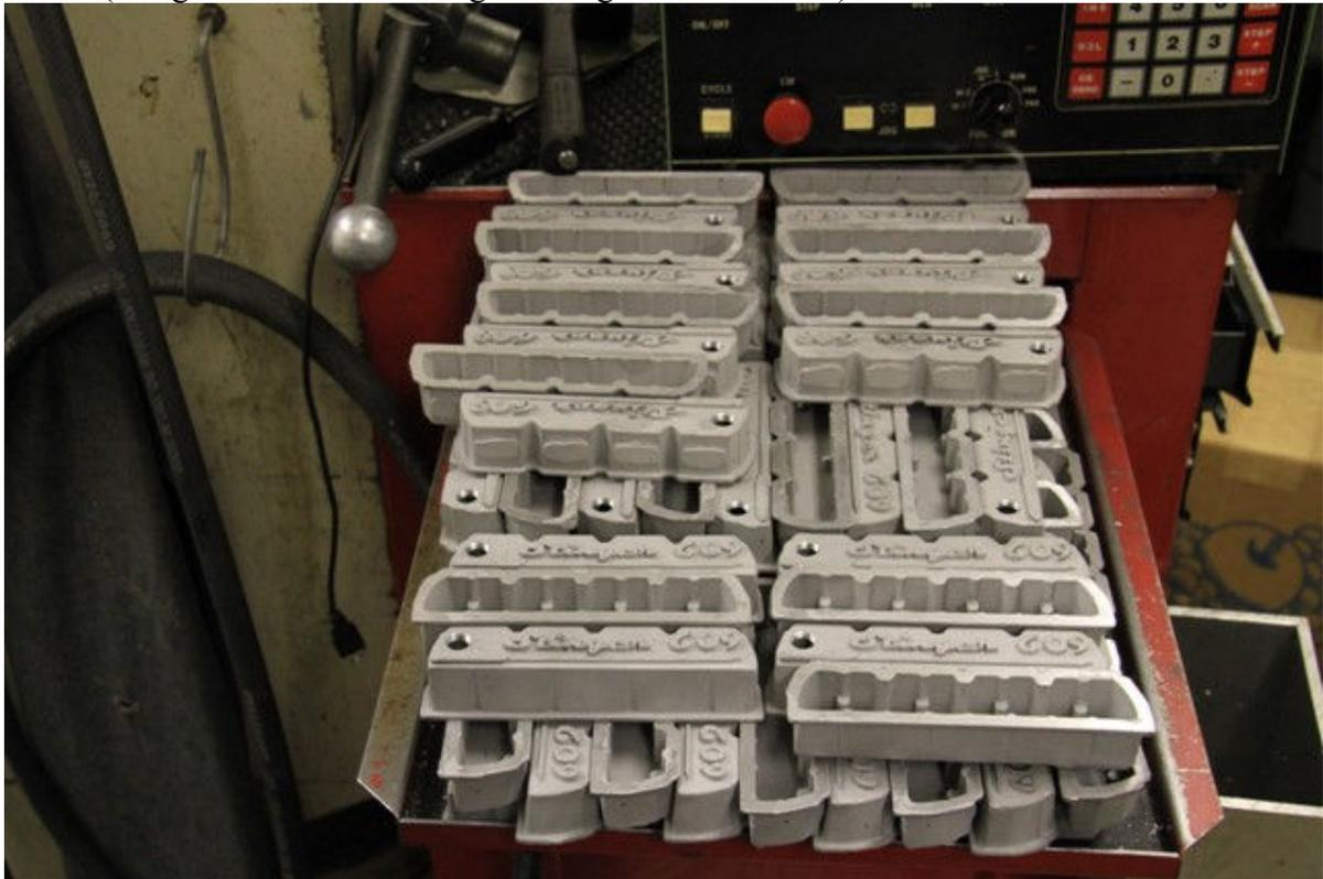
Pic #6 (Pieces of new starter motor gear case)
