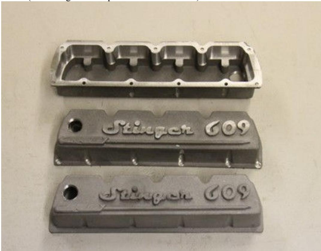
Pic #5 (Rough valve cover castings waiting to be machined)
