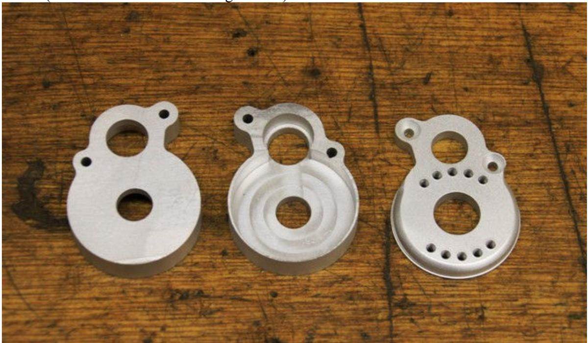
Pic #7 (Completed starter motor gear case halves)
