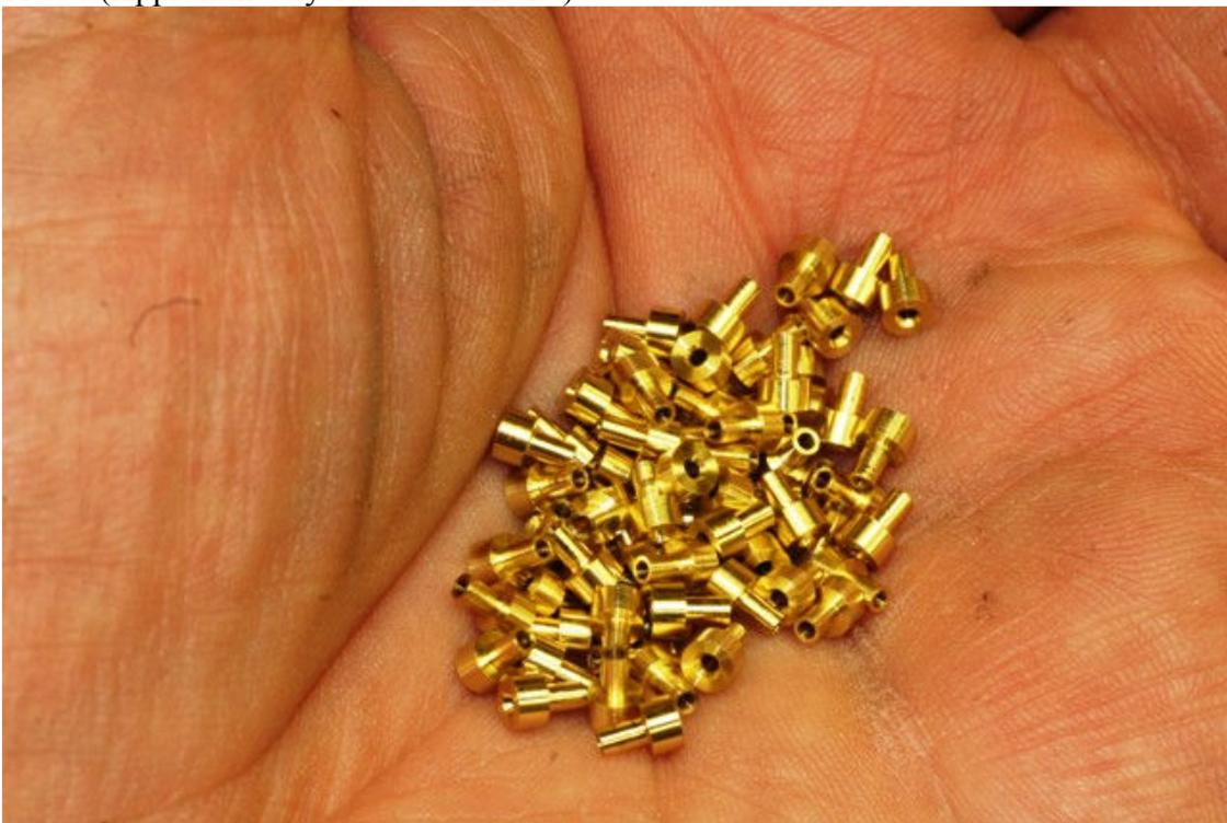
Pic #5 (Hollow dowel pin to keep main bearing from spinning)
