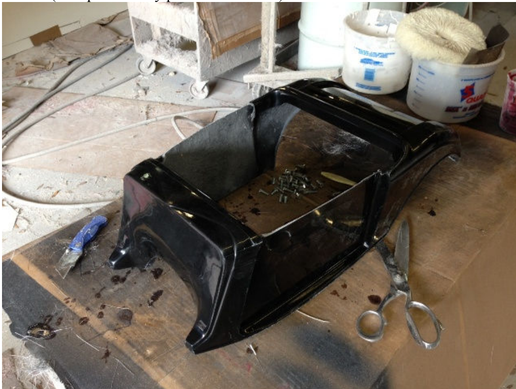
Pic # 6 (Completed body pulled from mold)
