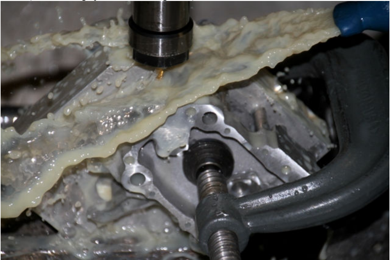
Pic #8 (3 rd machining operation on timing cover)
