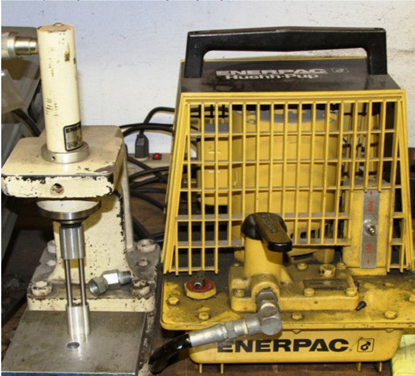
Pic #13 (Hydraulic press used assemble supercharger impellers)
