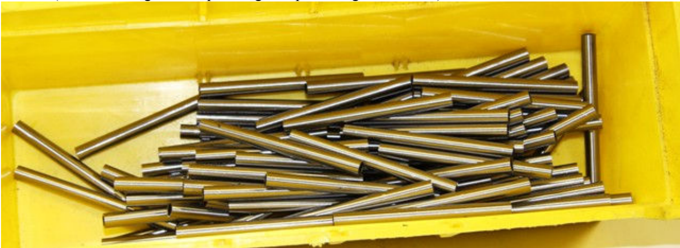
Pic #10 (Finished and ground supercharger impeller alignment tubes)
