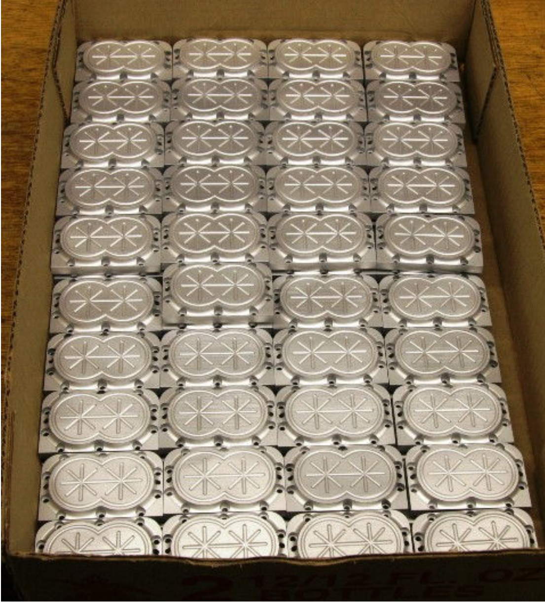
Pic #13 (Finished and glass beaded rear plates)
