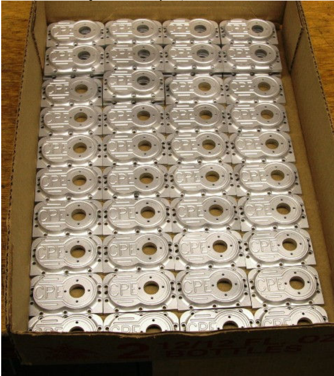
Pic #12 (Finished and glass beaded front plates)
