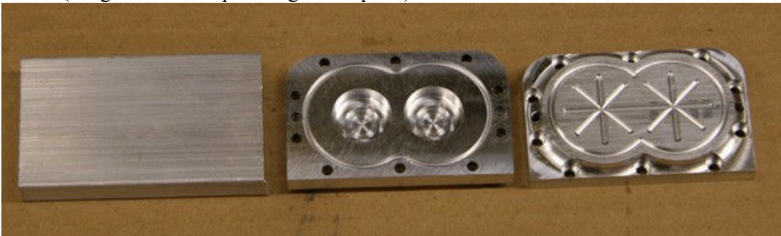
Pic #9 (Progression of supercharger rear plate)
