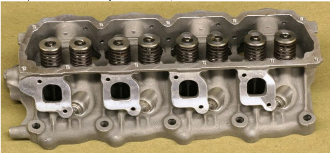
Pic #4 (Assembled head ready for installation)
