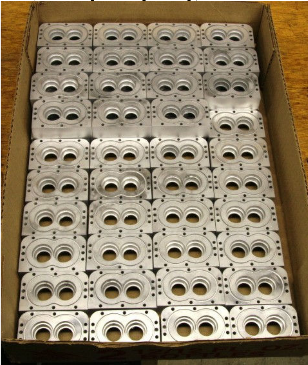
Pic #11 (Finished and glass beaded gear housings)
