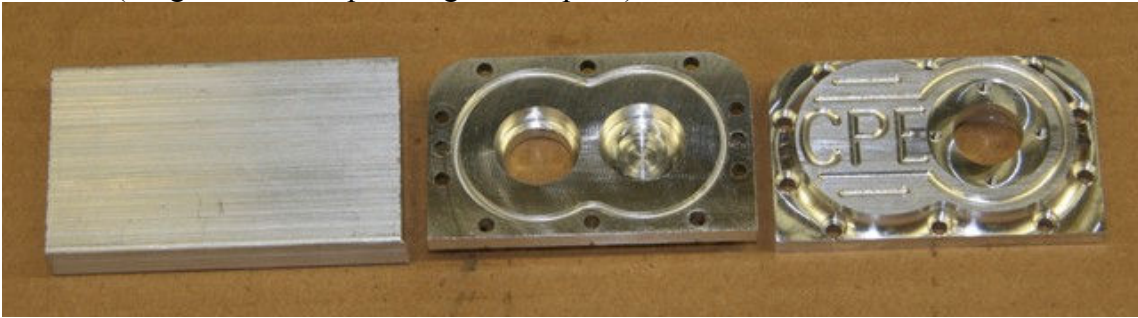
Pic #11 (Finished and glass beaded gear housings)
