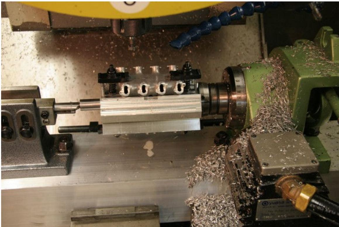
Pic #3 (Keyway cutter machining bottom – inside edge of leg on intake manifold)
