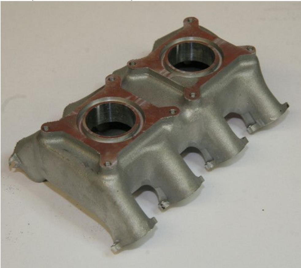
Pic # 5 (Finished intake manifold)
