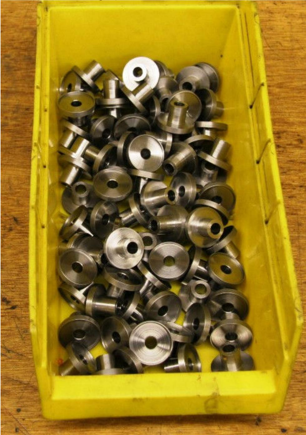
Pic #8 (Supercharger impeller alignment tubes)
