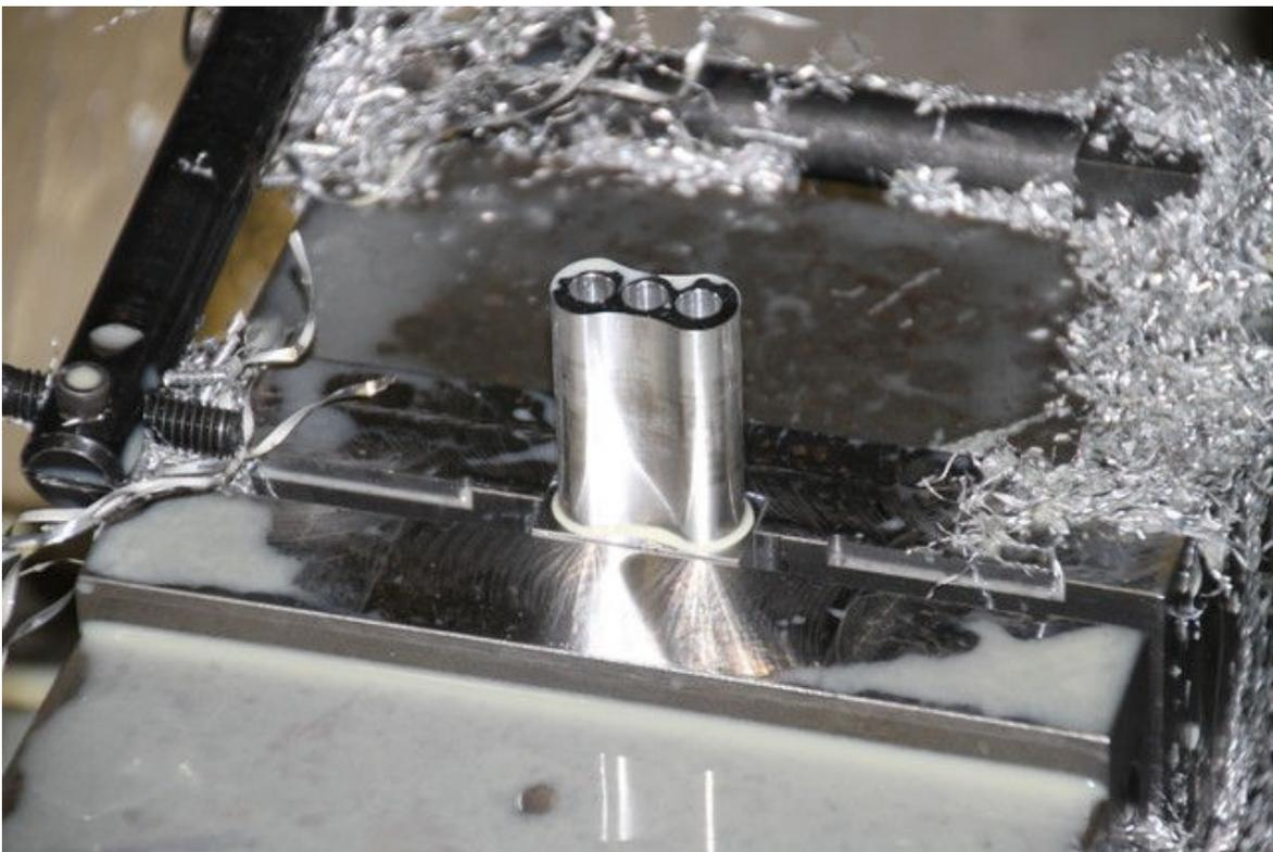
Pic #5 (Completed impeller halves ready for further machining)
