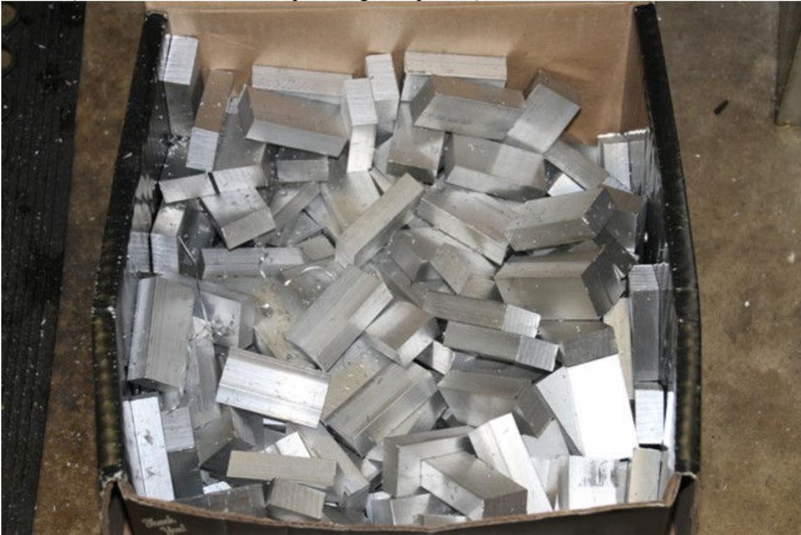
Pic #2 (Blank ready for machining)
