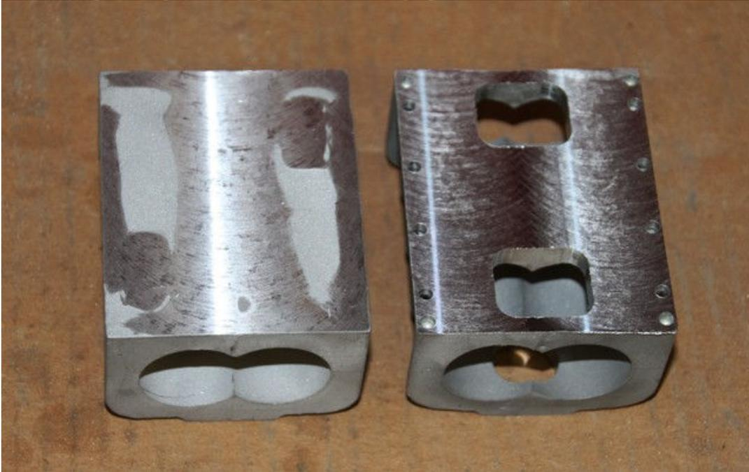
Pic #10 (Supercharger housing, second machining operation)
