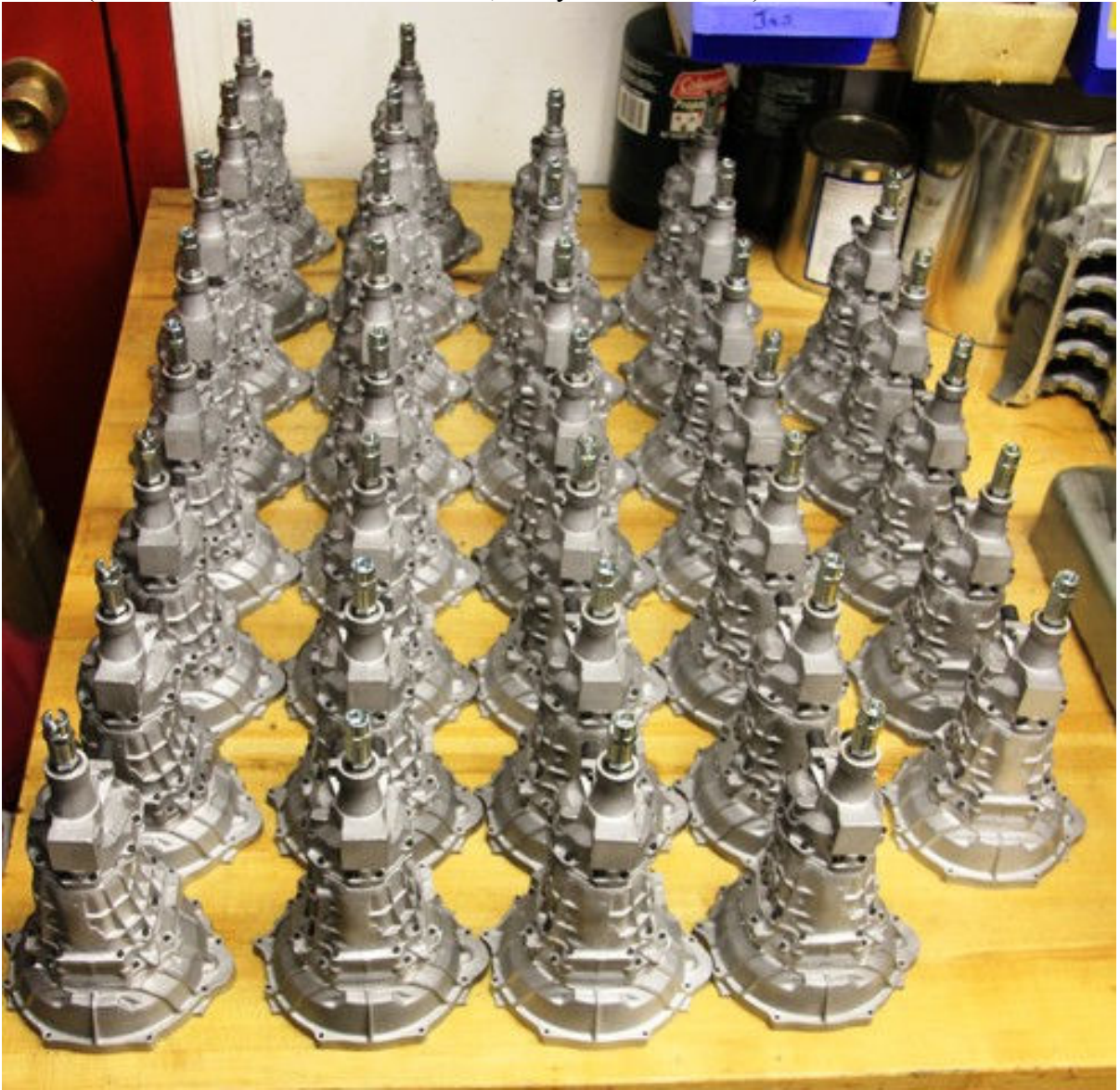
Pic #1 (Finished transmission assemblies, ready for installation)
