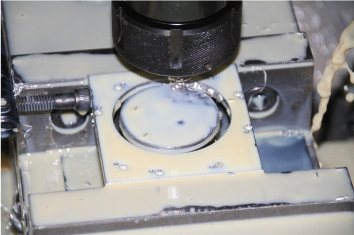
Pic #4 (Completely machined transmission adaptor plates)
