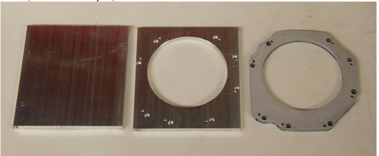
Pic #3 (Circular Interpolation of transmission adaptor)
