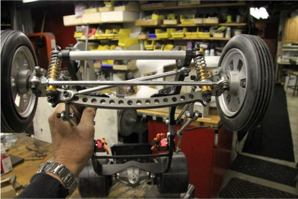
Pic #8 (Bottom view of installed quick change rearend)
