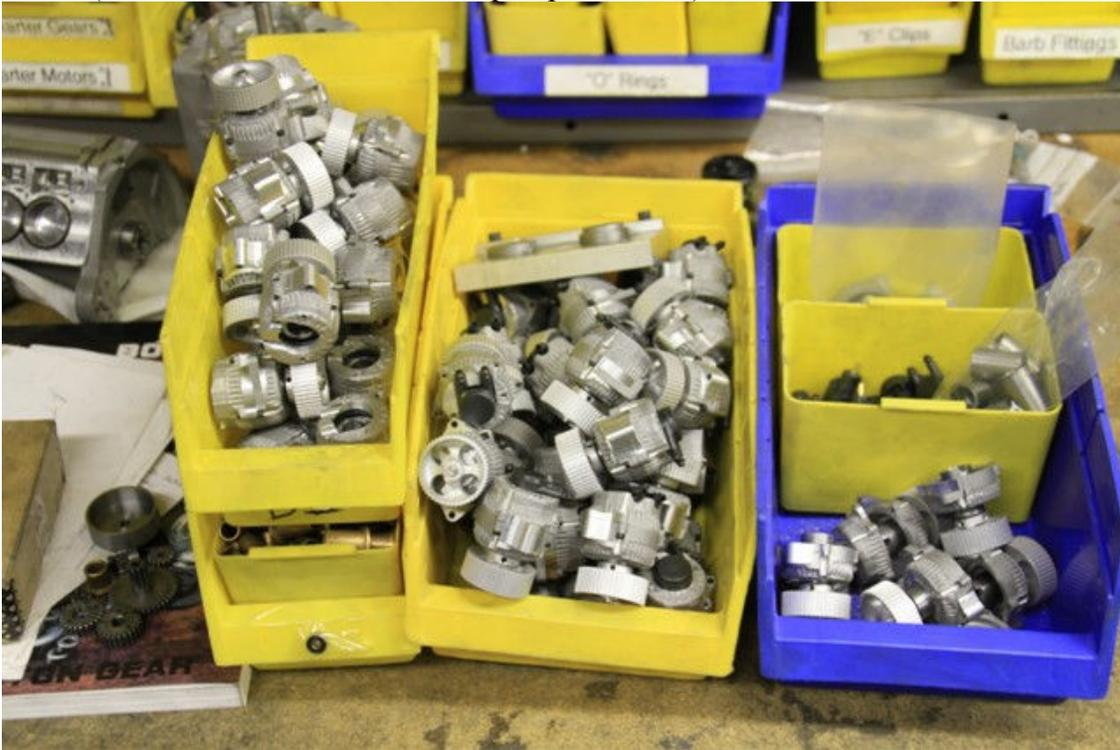
Pic #3 (Supercharger impellers ready for assembly)
