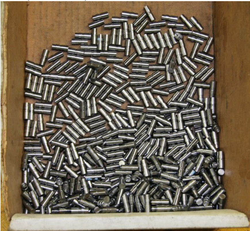
Pic #3 (Finished lifters)
