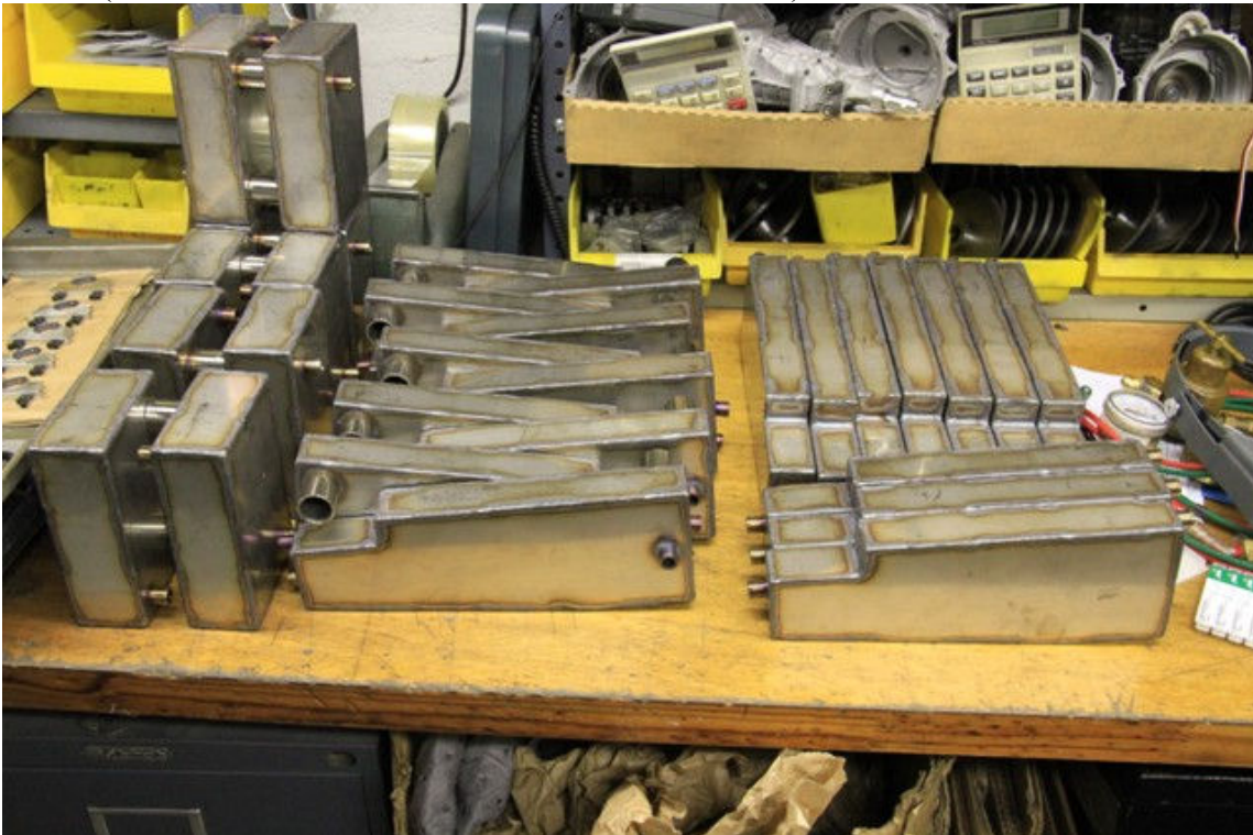
Pic #8 (Stainless steel water and oil tanks for test stands)
