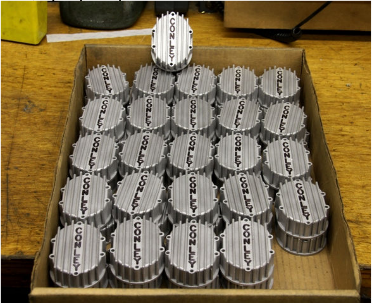
Pic #10 (Completed quick change rearend back covers)
