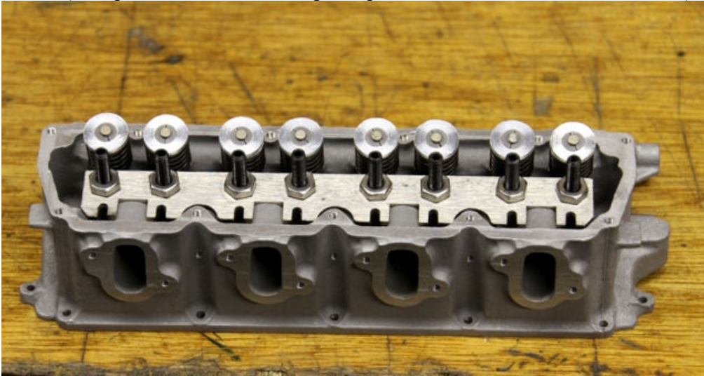
Pic #9 (Completed head with new guide plate and rocker arm studs installed)
