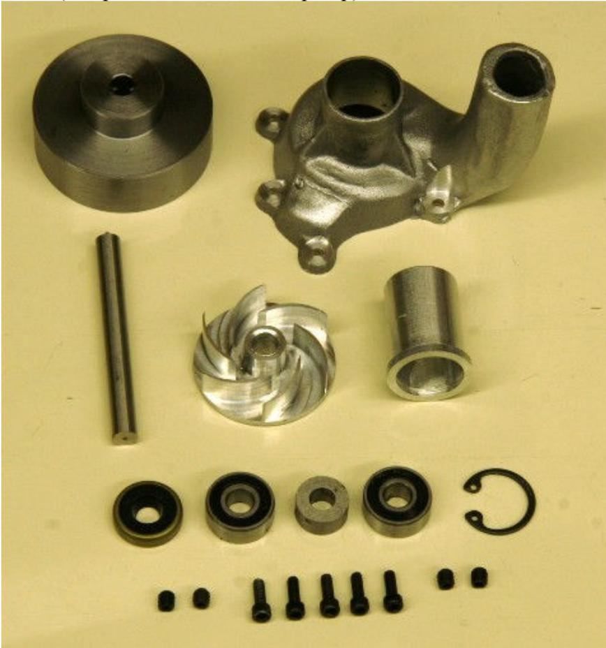
Pic #9 (water pump bearing and seal support)
