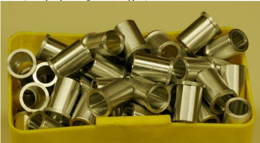
Pic #10(water pump bearing and seal support)
