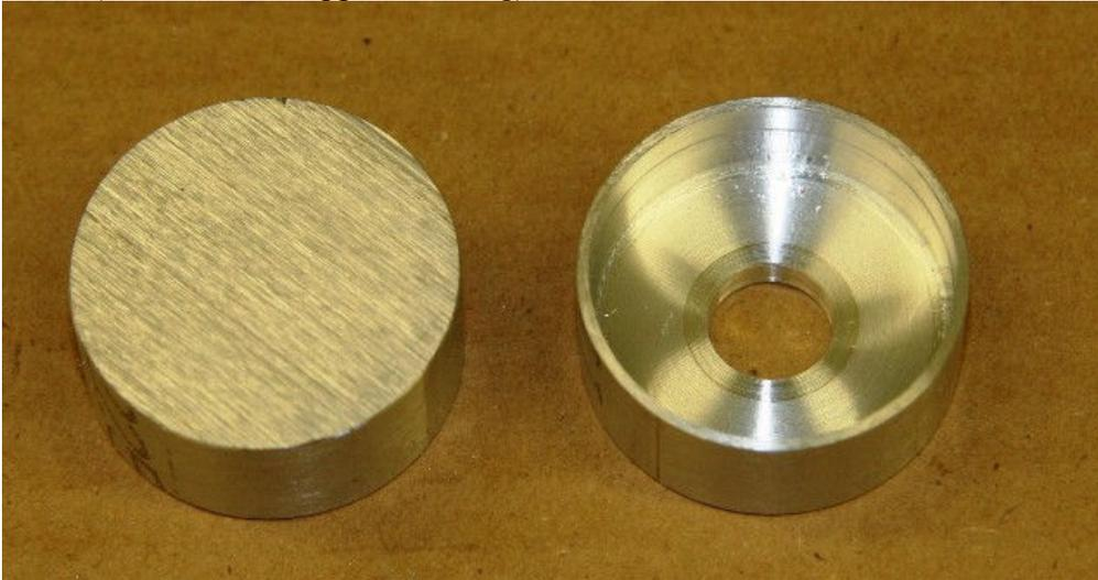
Pic #5 (finished starter motor support housings)
