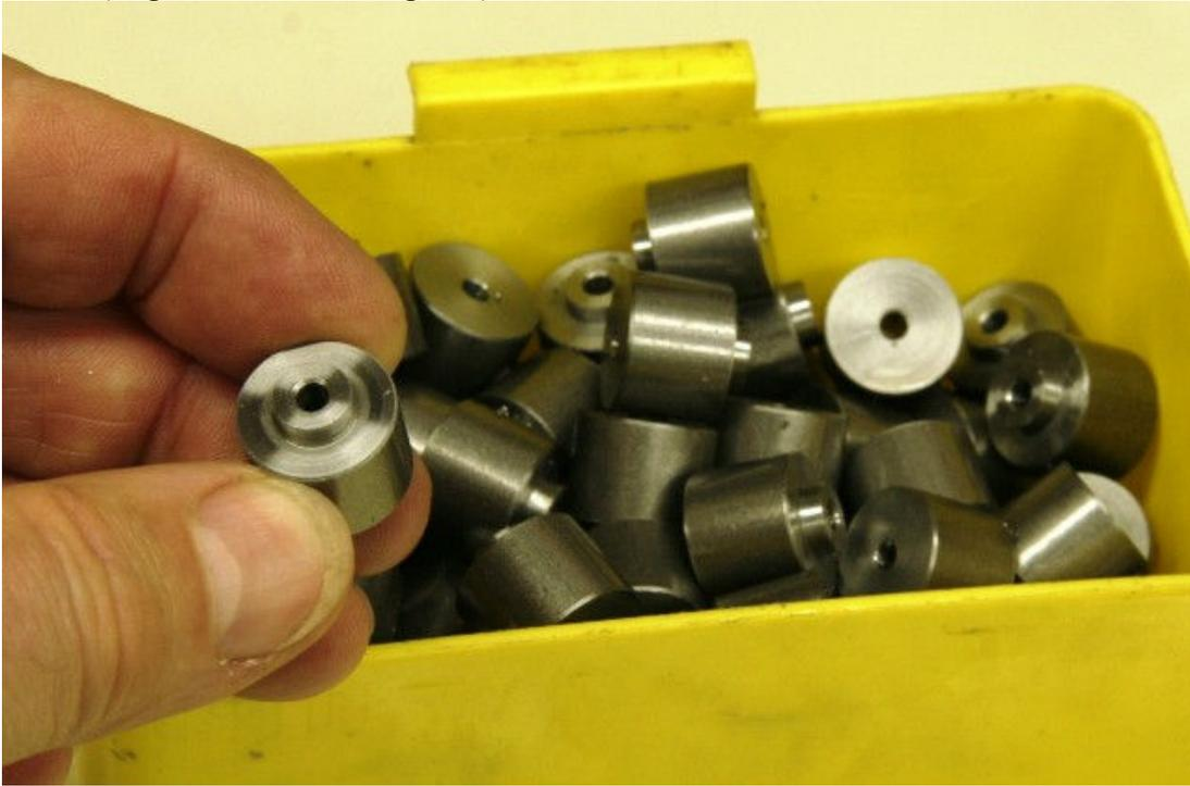
Pic #17(special collets needed to machine all the round parts)
