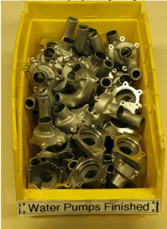
Pic #7(finished water pump housing)
