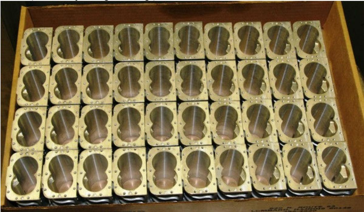
Pic #2 (rough supercharger housing casting)
