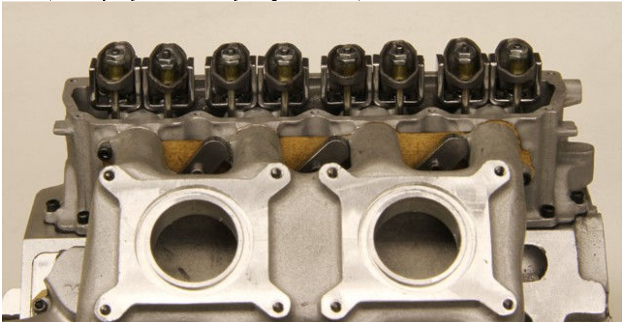
Pic #1 (Older style “jam” nuts for adjusting rocker arms)
