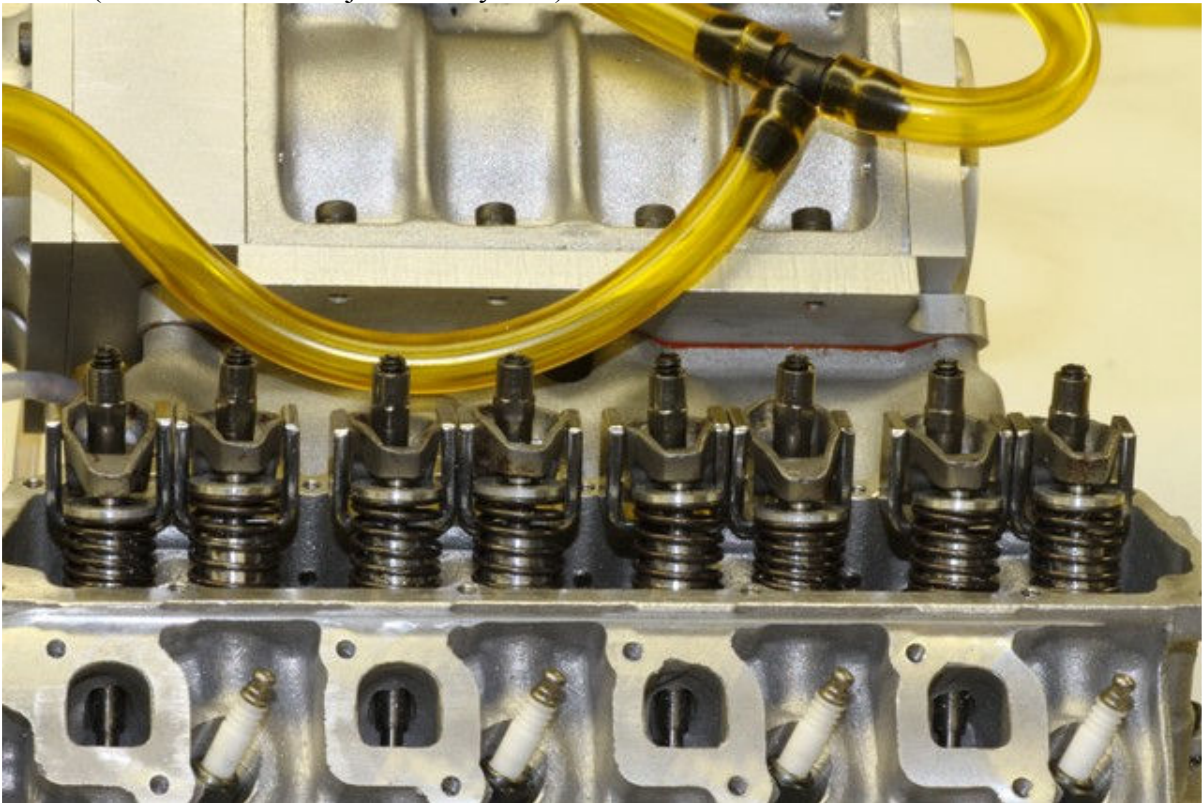
Pic #3 (Close-up of new rocker arm adjustment system)
