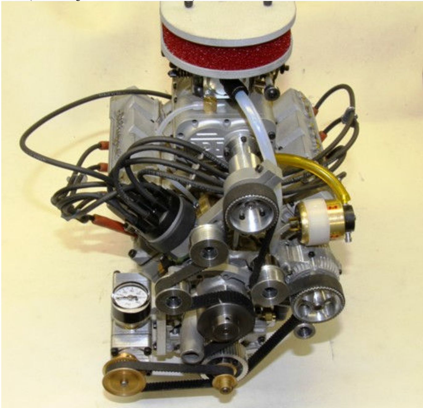
Pic #7 (Front of engine with distributor installed)
