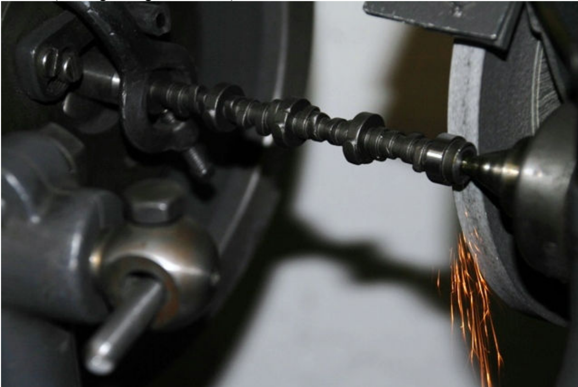
Pic #11 (Initial grinding of camshaft)
