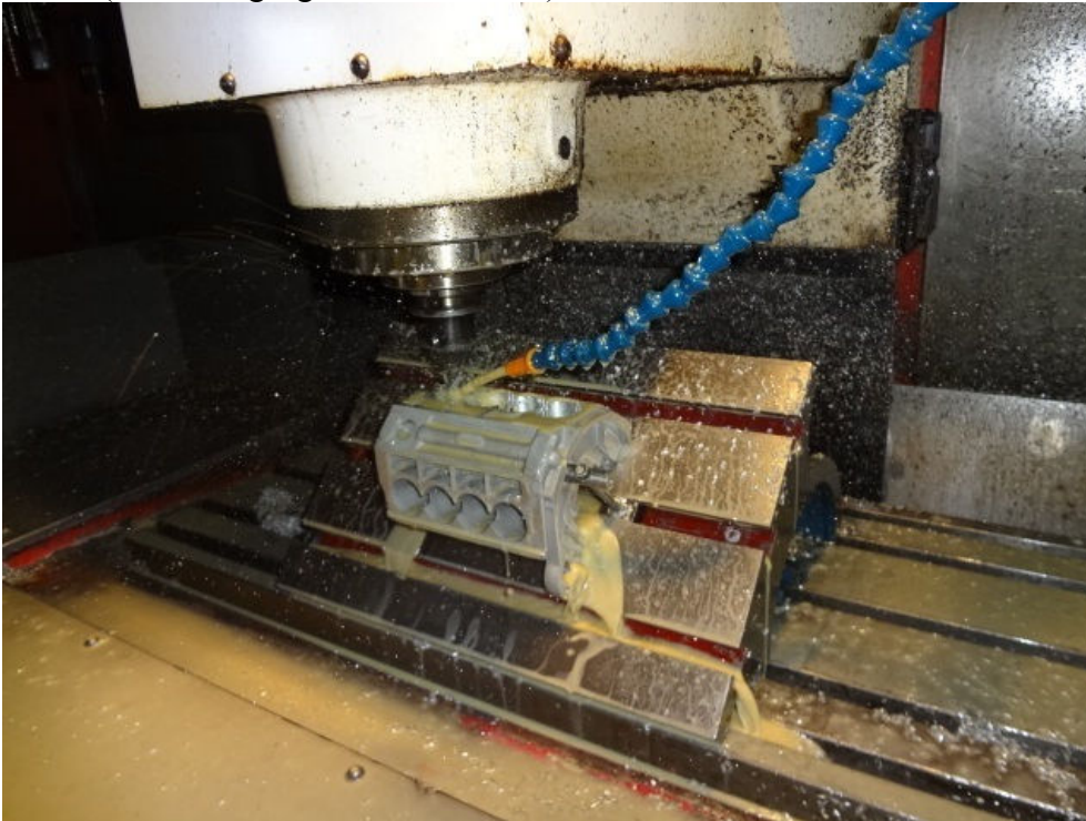
Pic #1 (Machining right bank of block)
