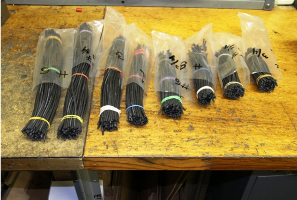
Pic #10 (Spark plug wire cut and ready for installation)
