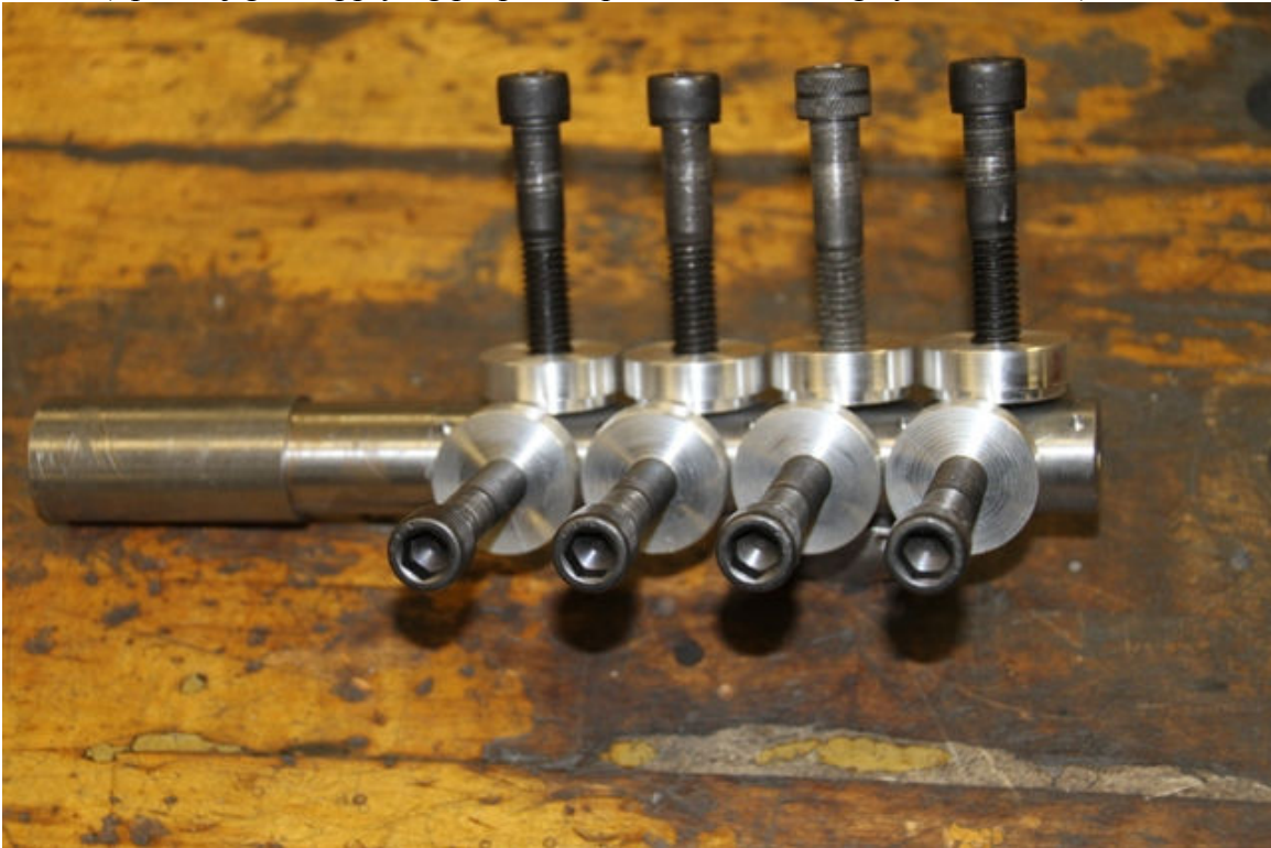
Pic #2 (Special jig for applying proper torque when installing cylinder liners)
