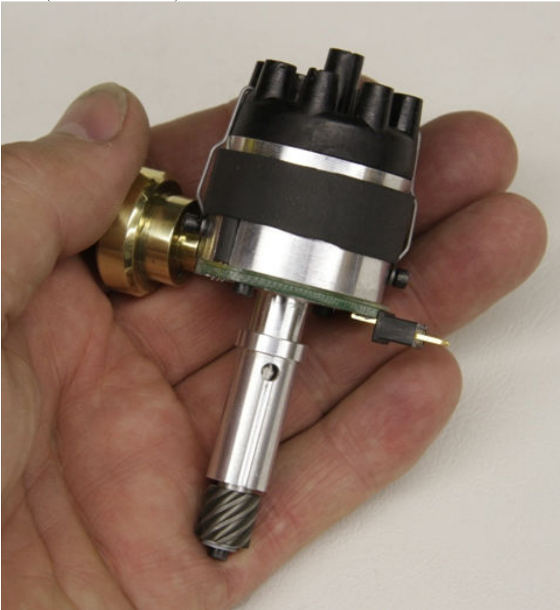
Pic #1 (Finished distributor)
