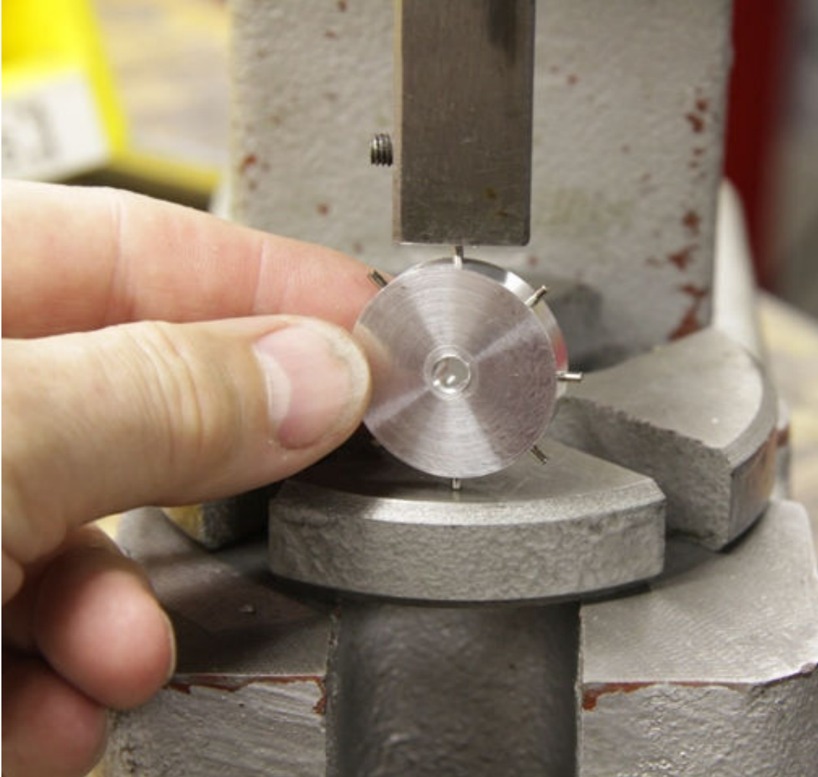
Pic #11 (Pressing magnets into aluminum rotor)
