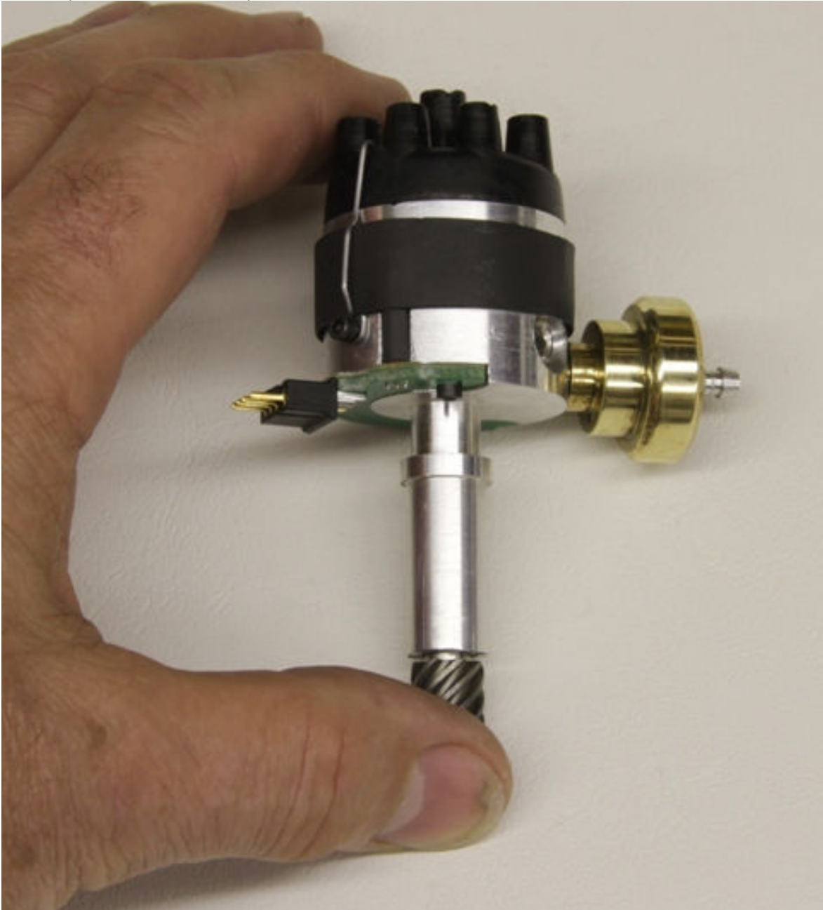
Pic #3 (Finished distributor)
