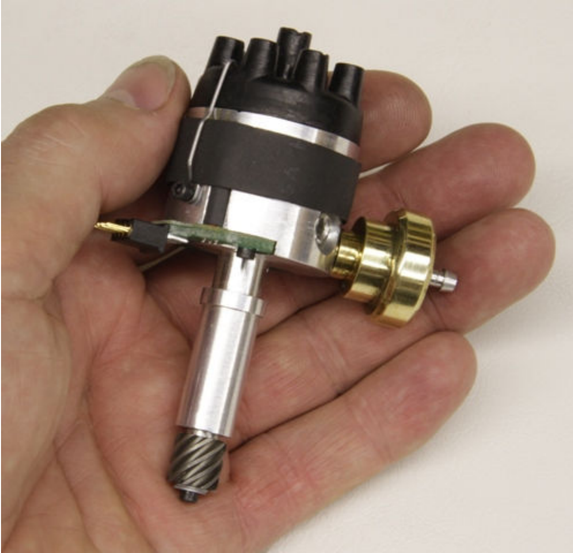
Pic #2 (Finished distributor)
