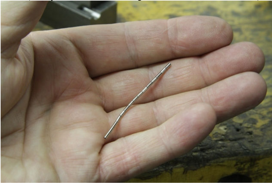
Pic #10 (Individual Neodymium-Iron-Boron magnet .062 dia. x .125 length)
