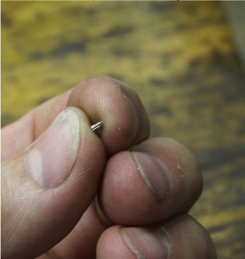
Pic #10 (Individual Neodymium-Iron-Boron magnet .062 dia. x .125 length)
