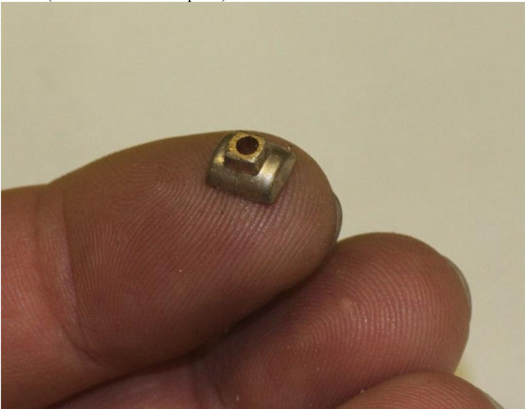
Pic #6 (Completed first operation on "Toggle" clamps for intake manifold)
