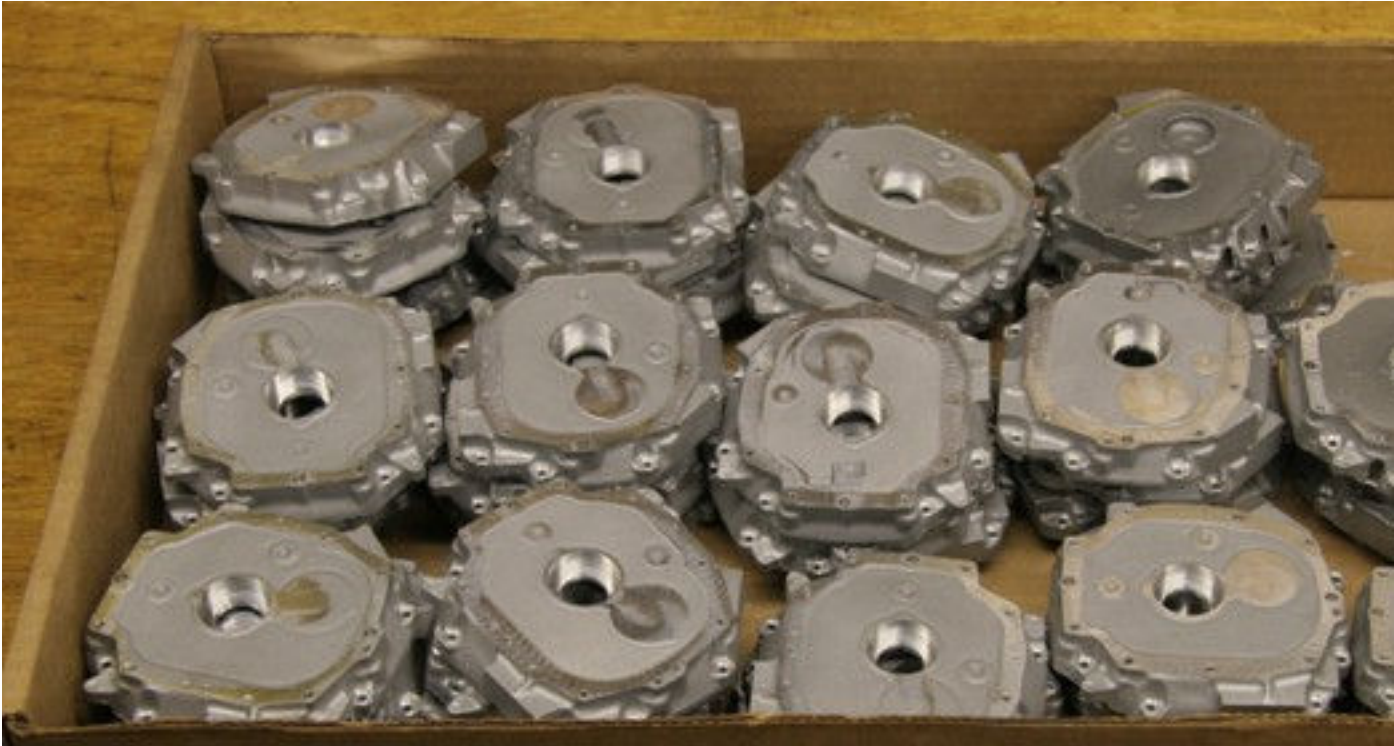
Pic #3 (Finished transmission adaptor plates)
