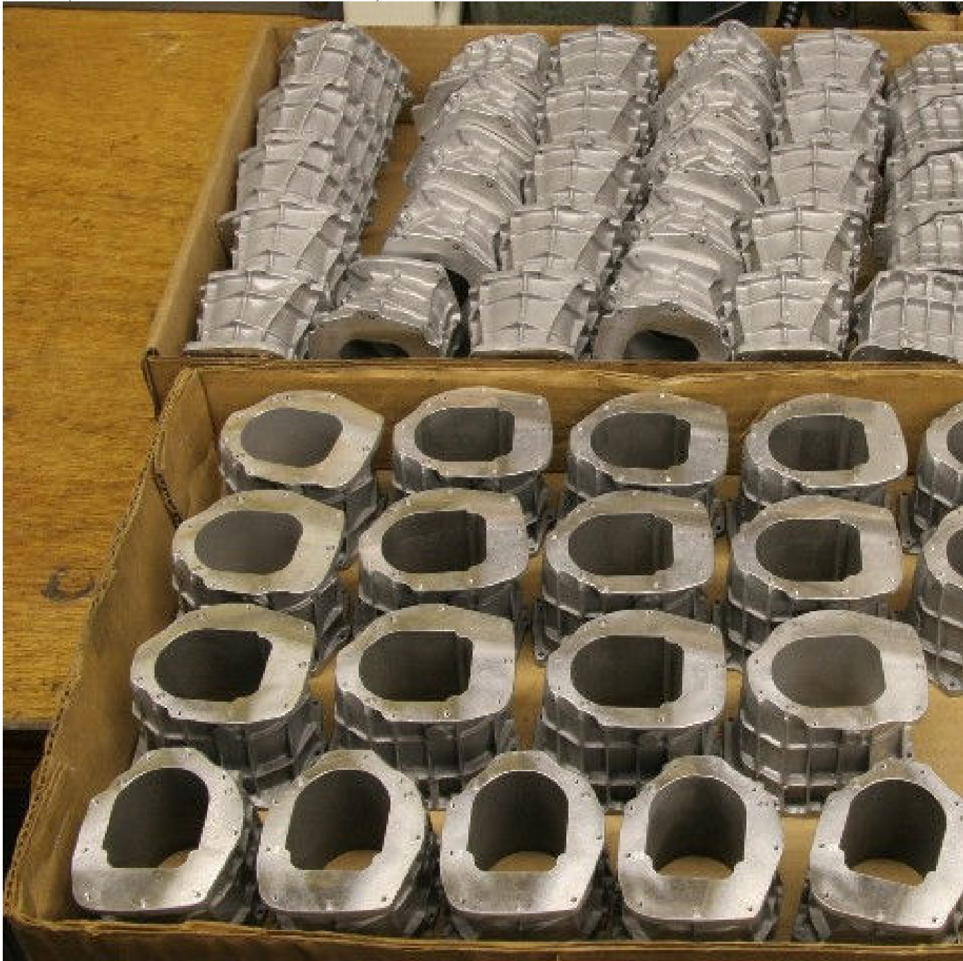
Pic #5 (Finished transmission center cases)
