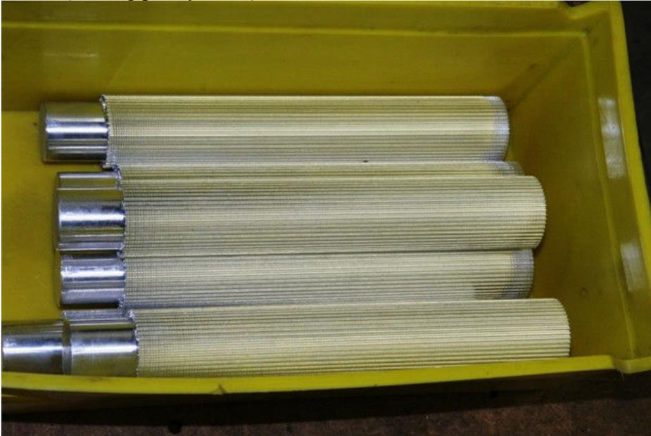
Pic #9 (Timing pulley stock cut into lengths)
