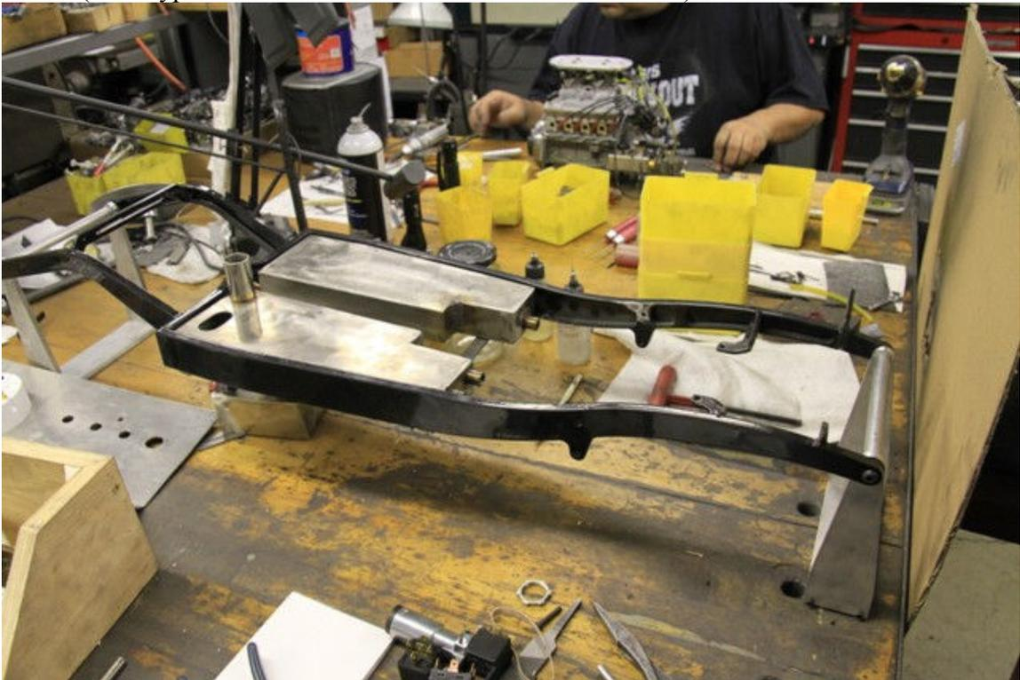
Pic #4 (Prototype test stand with basic engine installed to check placement & alignment)
