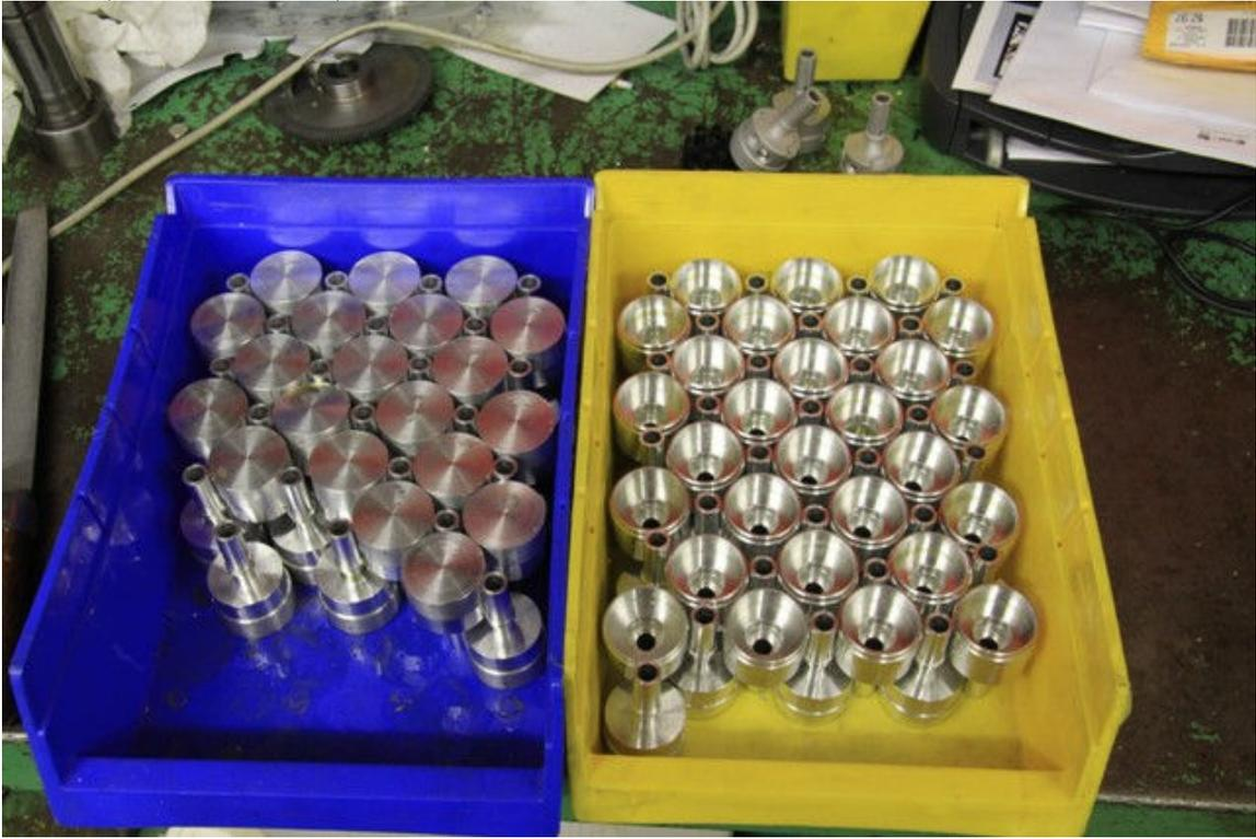
Pic #8 (Distributor machining operation)
