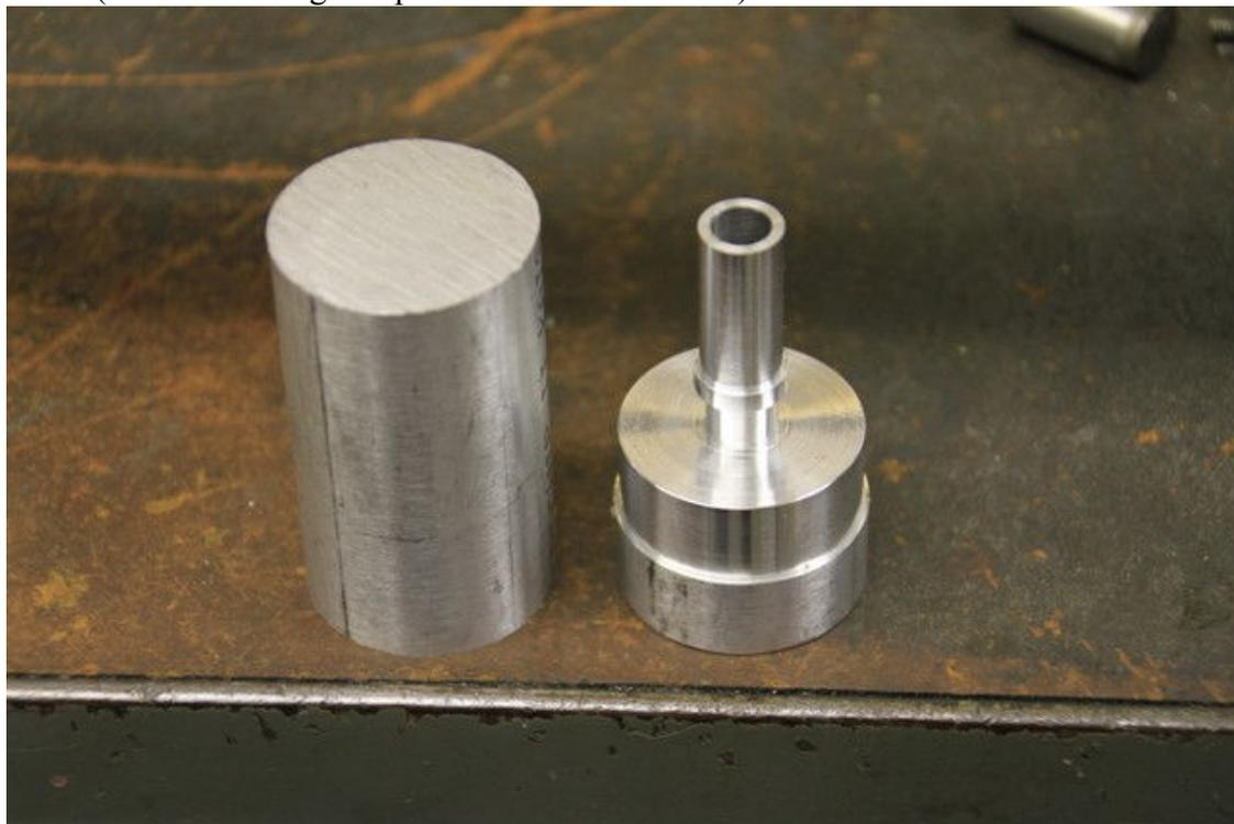
Pic #5 (Partially completed distributor, 1<sup>st</sup> operation)
