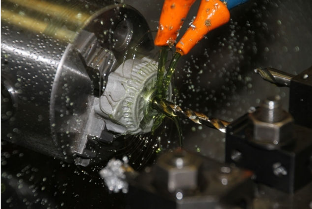
Pic #1 ( Initial machining operation for alternator halves)
