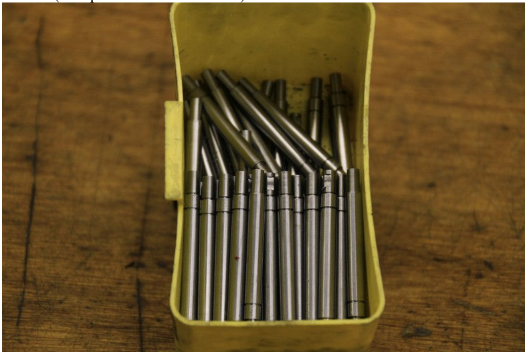
Pic #10 (Completed distributor shafts)
