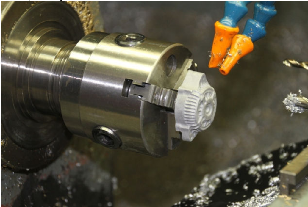
Pic #2 ( Holding fixture for alternator halves)
