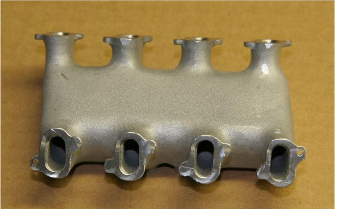
Pic #4 (Finished intake manifolds)
