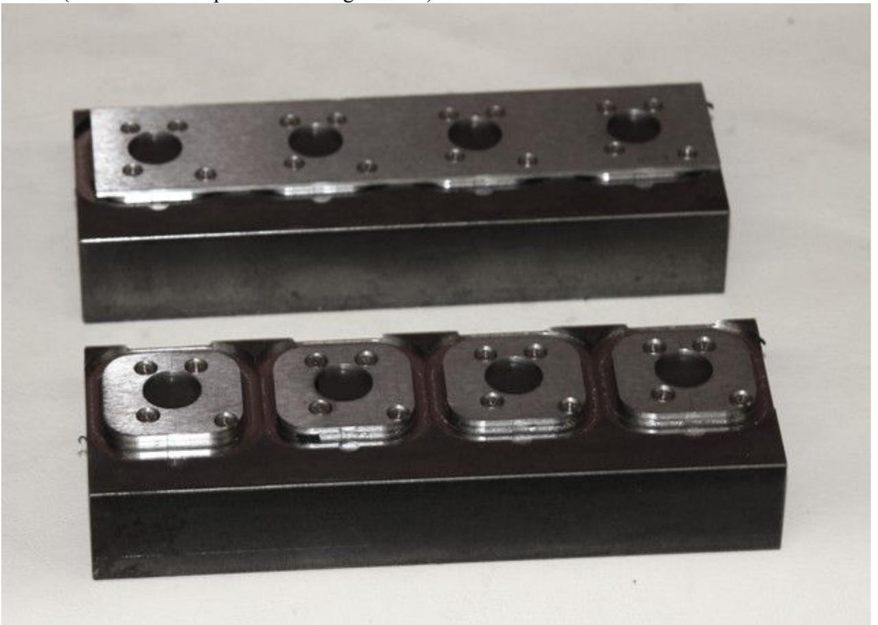
Pic #4 (Timing cover internal thrust plate)
