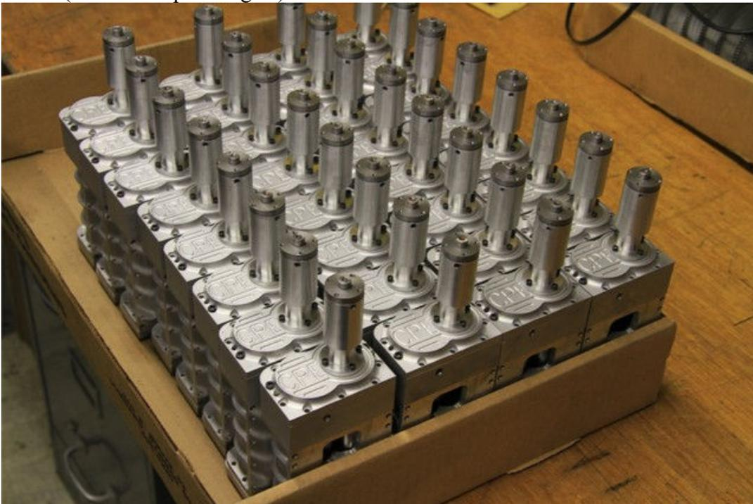
Pic #3 (Machining each cylinder to the exact height)
