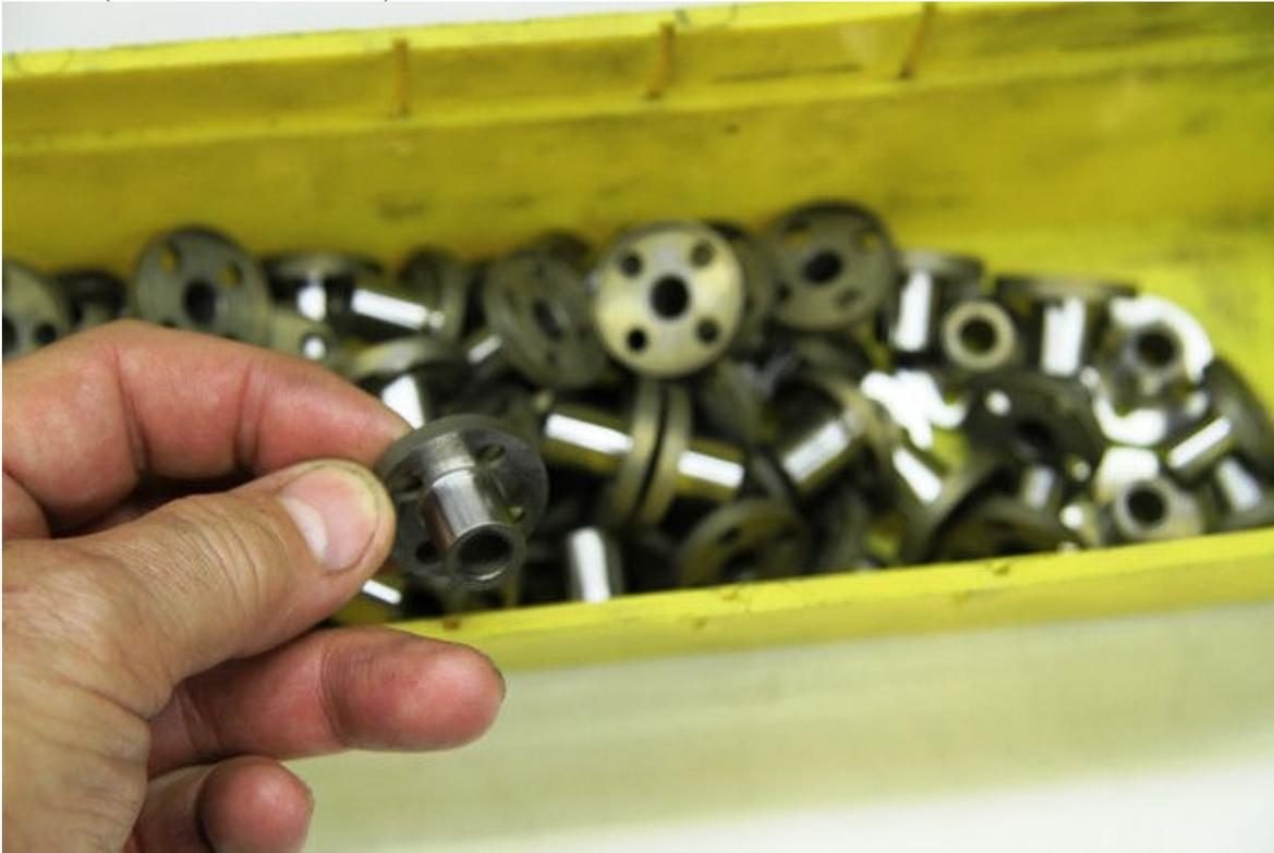
Pic #8 (Distributor drive shafts have been taped and fitted with gears)
