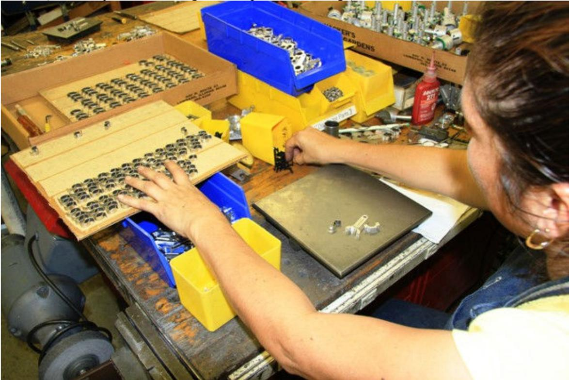
Pic #10 (Parts needed for each connecting rod)
