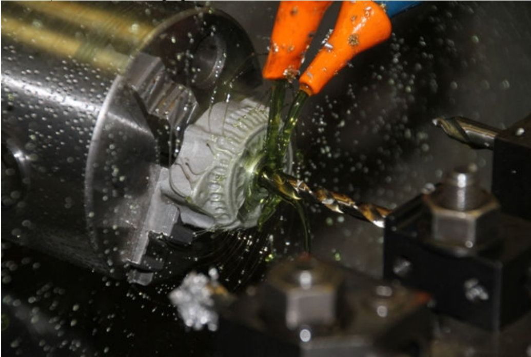
Pic #1 ( Initial machining operation for alternator halves)
