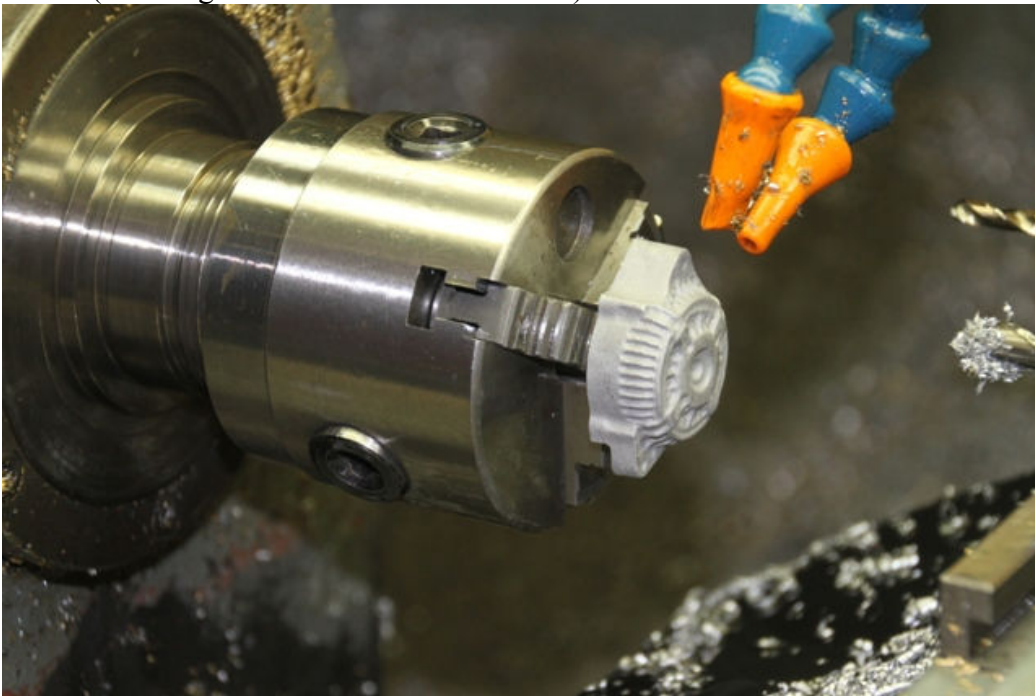
Pic #2 ( Holding fixture for alternator halves)
