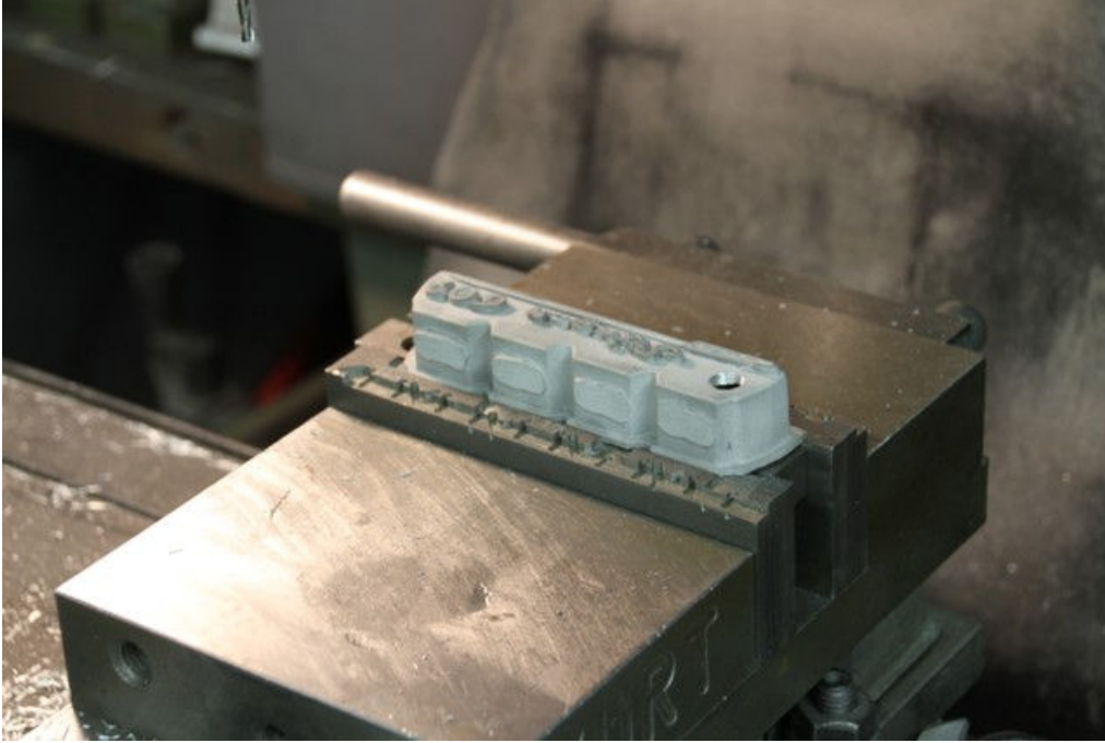
Pic #5 ( Unfinished valve cover before machining operations)
