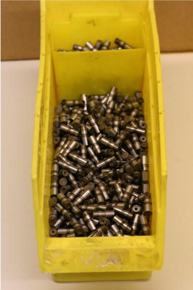
Pic #6(Water pump pulley blanks)
