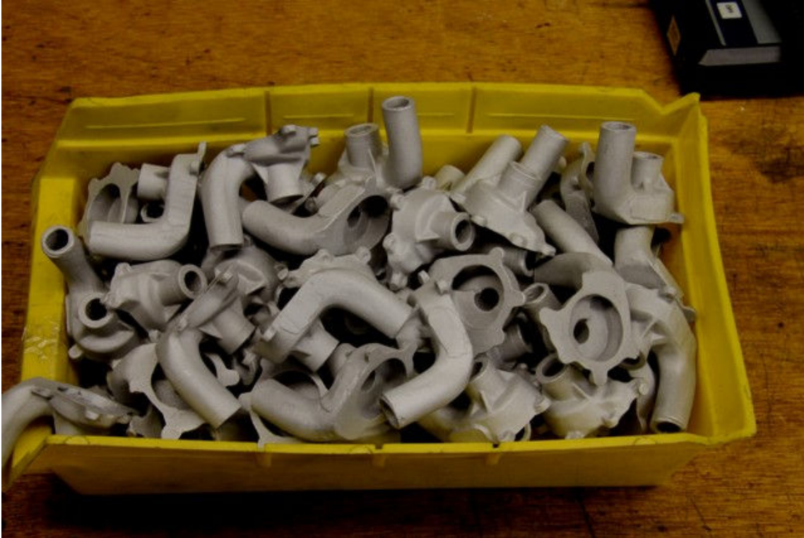
Pic #3 Water pump housing
