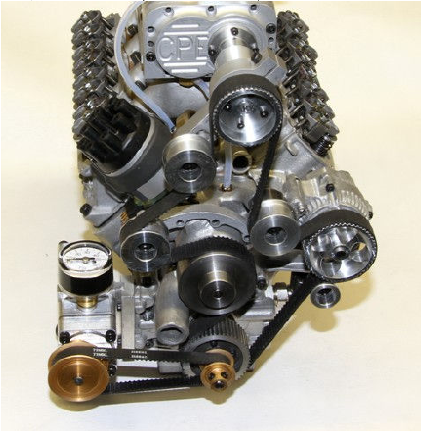
Pic #8 (Front view with new and improved idler bracket installed)
