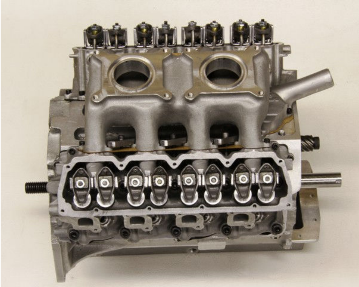
Pic #4 (Head showing rocker arms with guides and pushrod installed)
