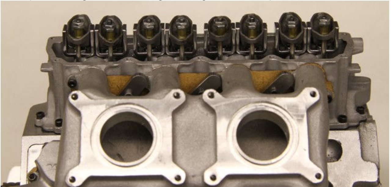
Pic #4 (Head showing rocker arms with guides and pushrod installed)
