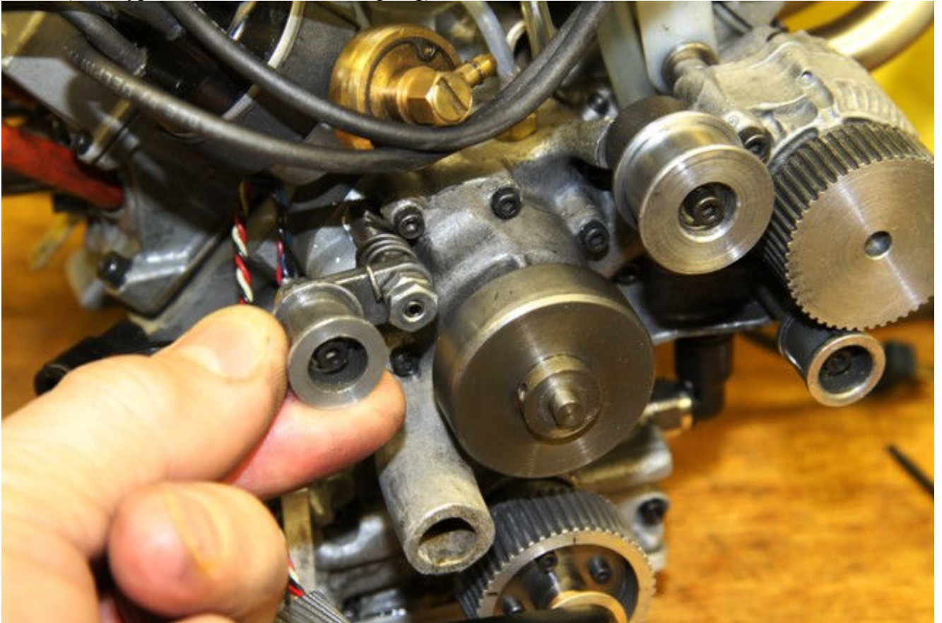
Pic #5 (Prototype idler with bracket and spring)
