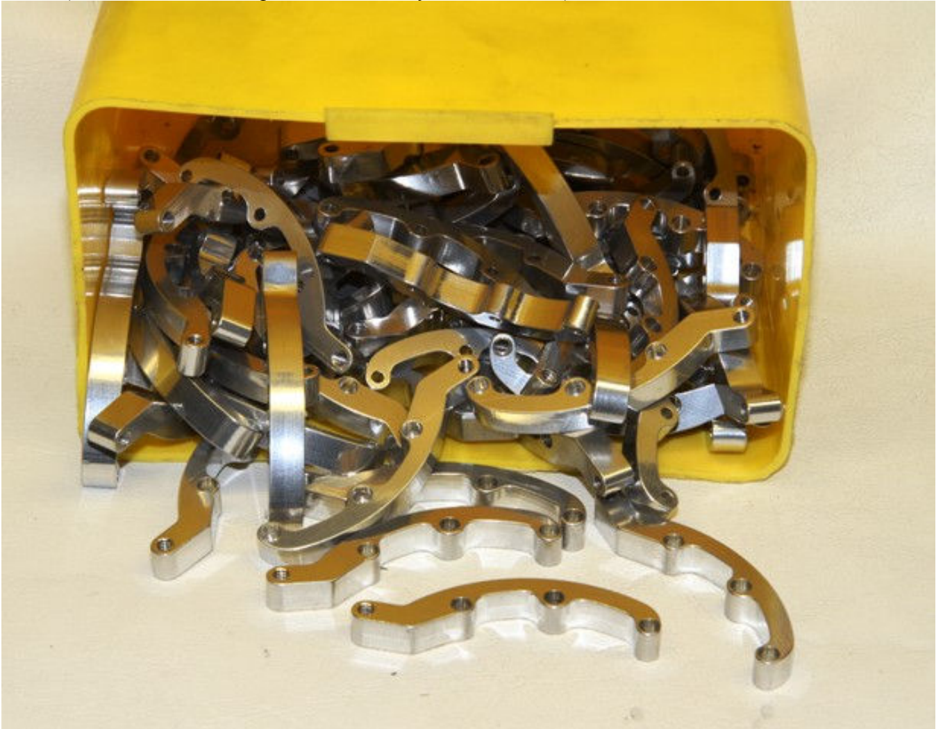
Pic #7 (New idler brackets – polished and ready for installation)
