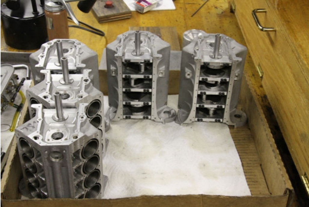
Pic #9 (Blocks with bearing halves and crankshafts installed)
