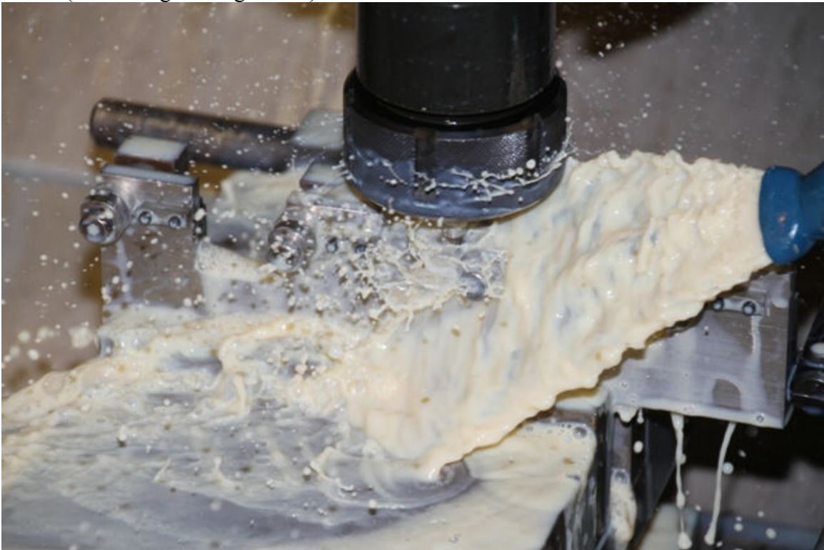
Pic #6 (Machining bearing halves)
