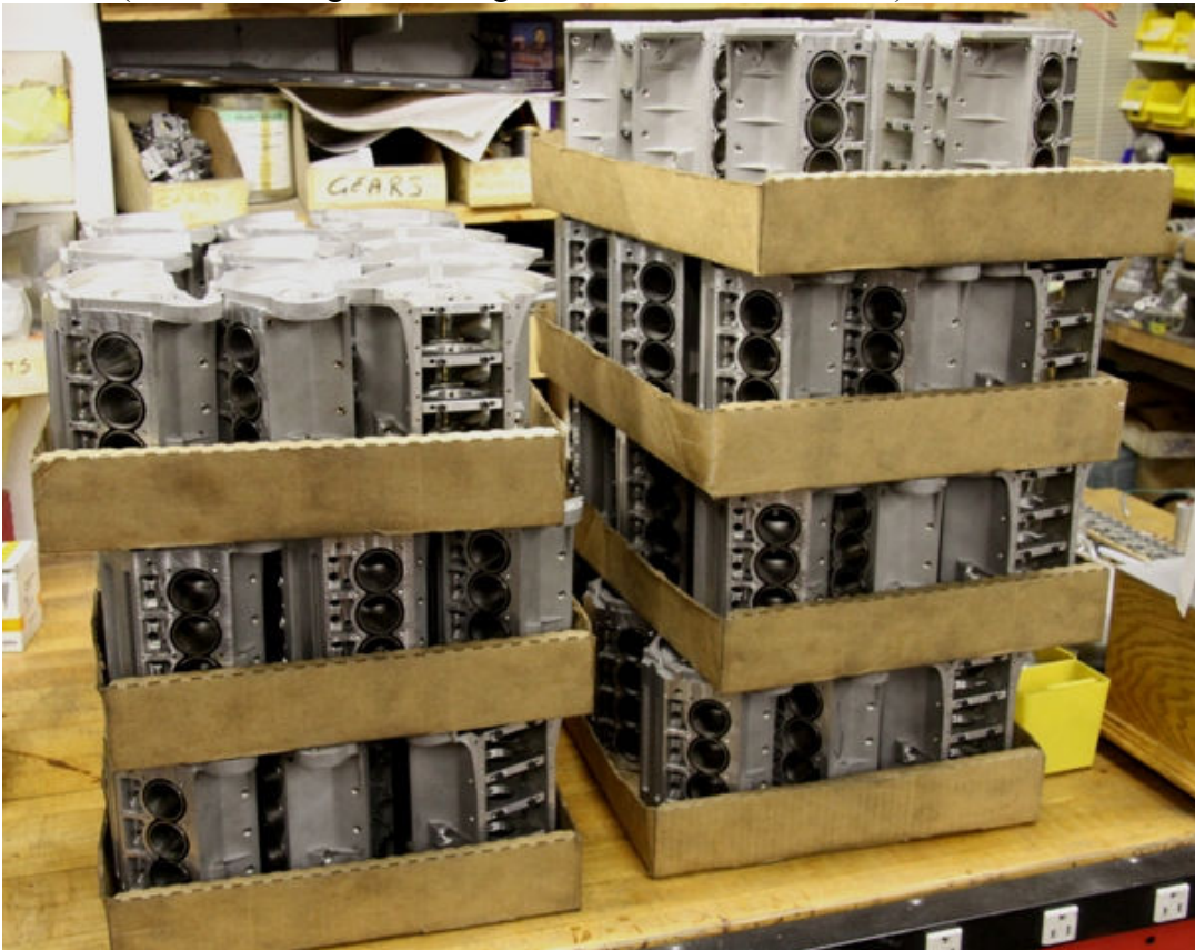
Pic #10 (Blocks waiting for bearing and crankshaft installation)
