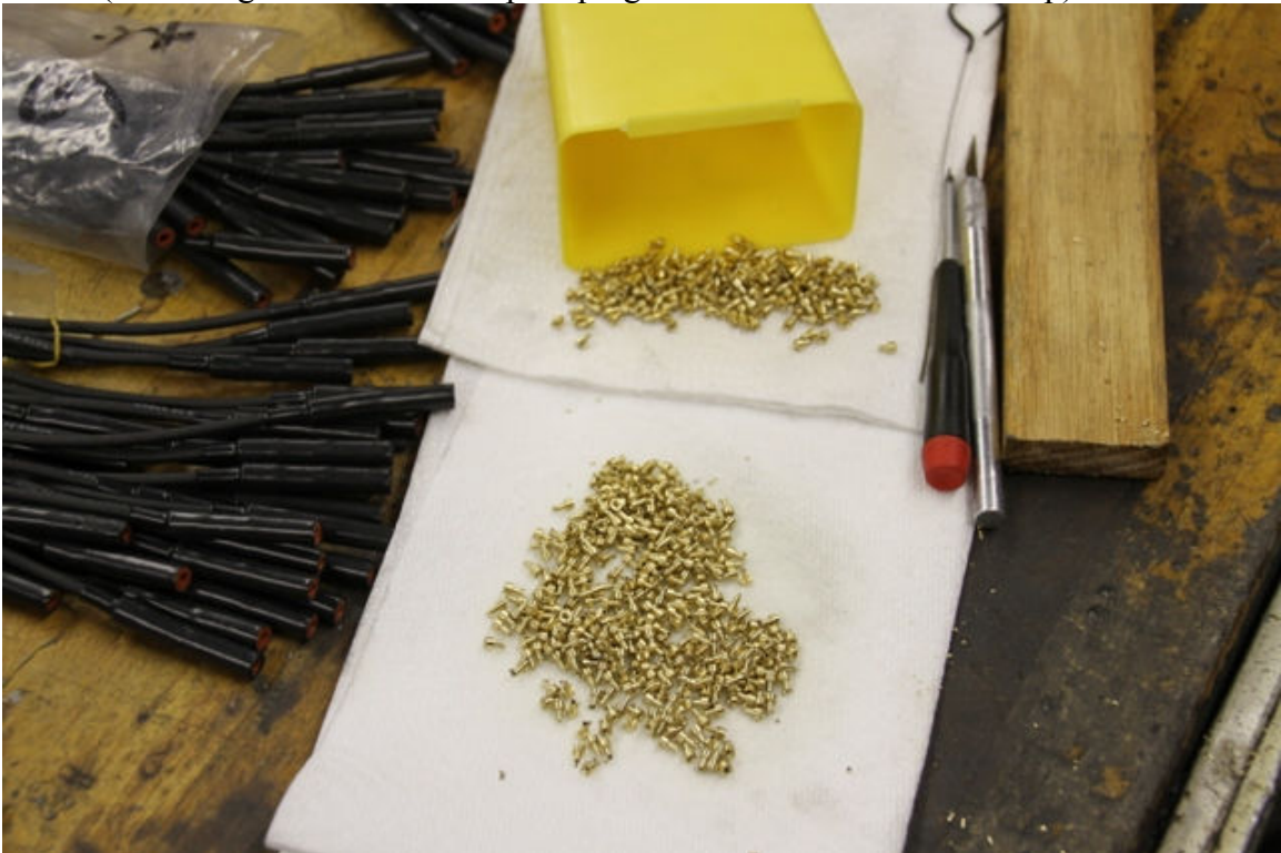
Pic #4 ( Installing brass inserts on spark plug wire then into distributor cap)
