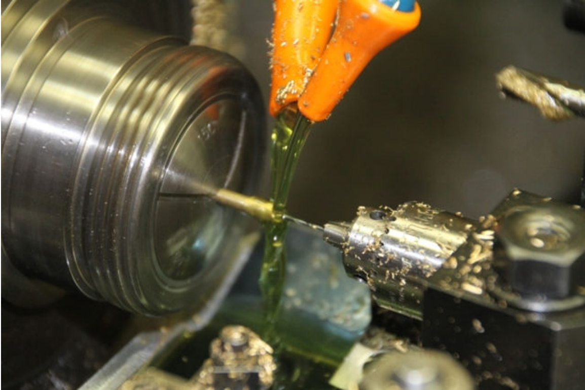
Pic #3 (Machining brass inserts for distributor cap)
