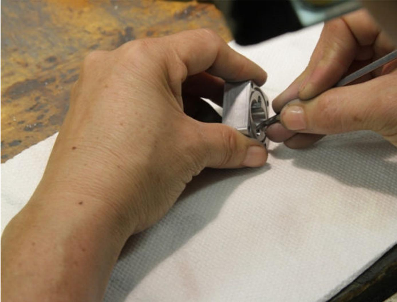
Pic #8 (De-burring oil pump housing)
