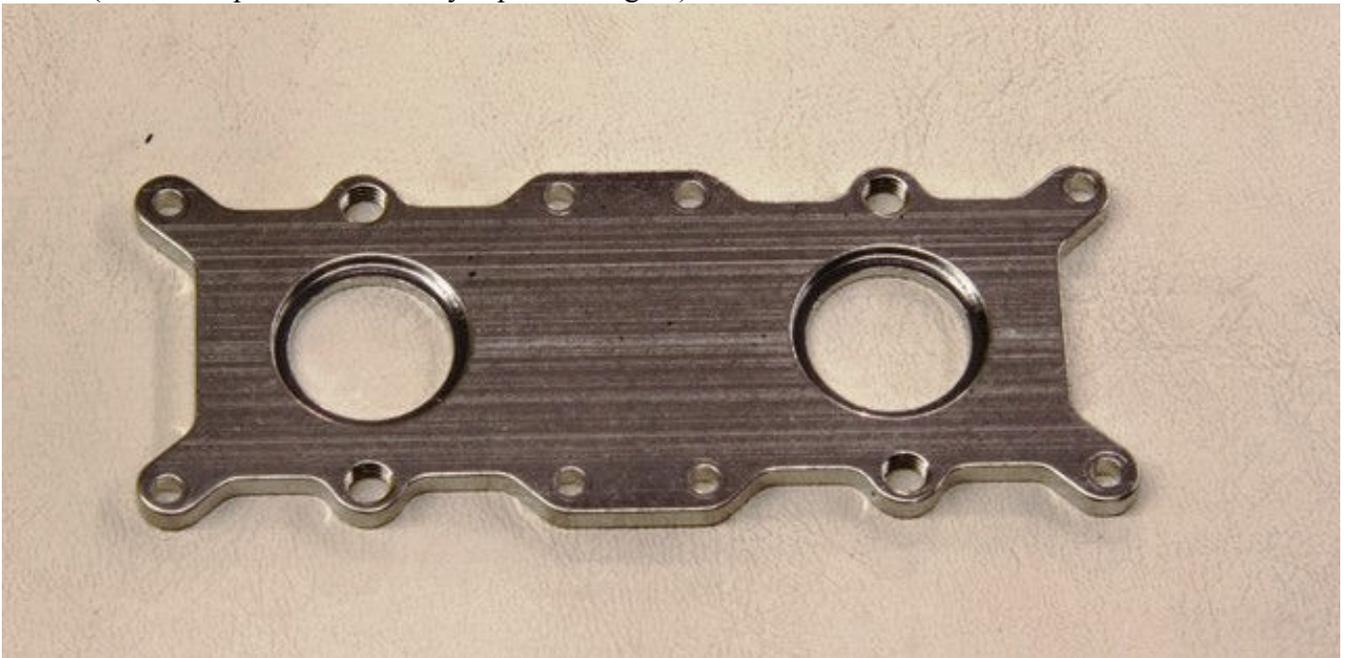
Pic #9 (Finished base plates for normally aspirated engine)
