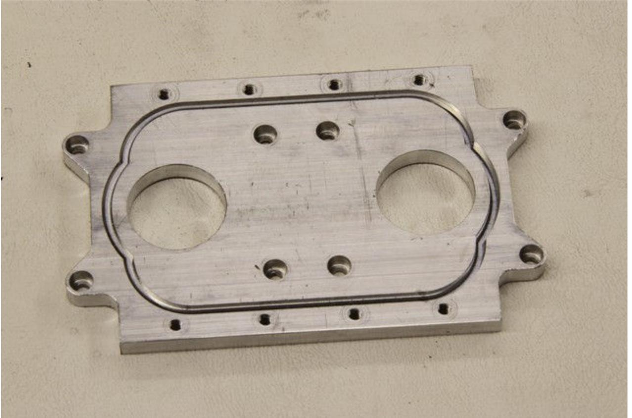
Pic #7 (Finished supercharger base plates)
