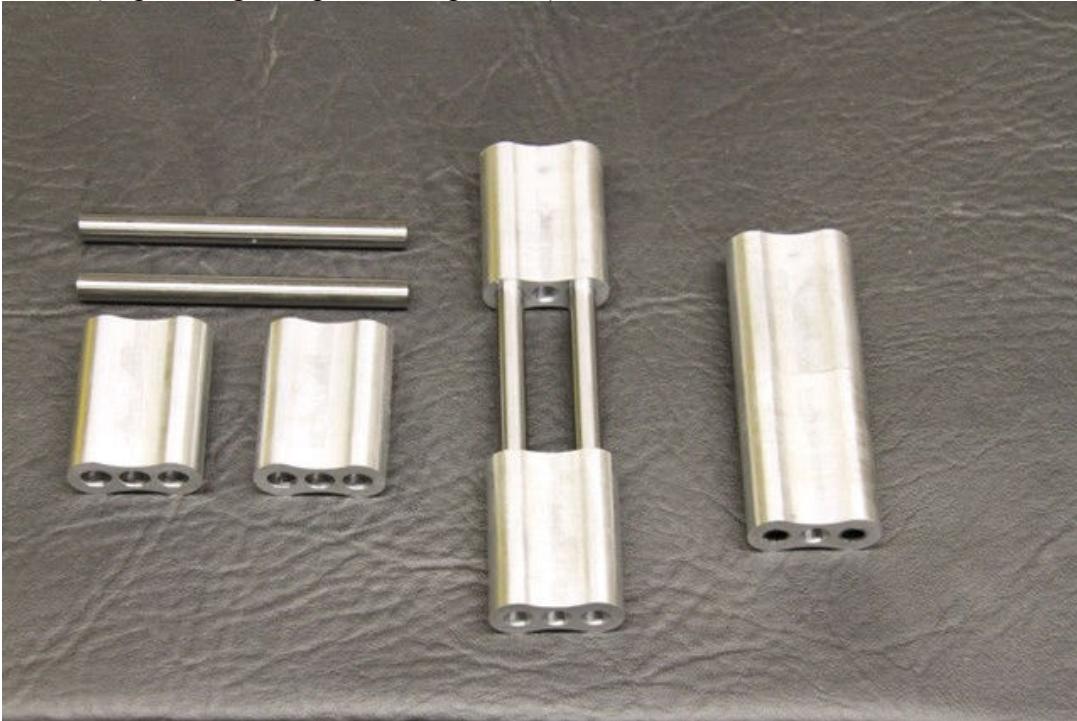
Pic #10 (Stainless Steel "Bung" for water tank and oil tank)
