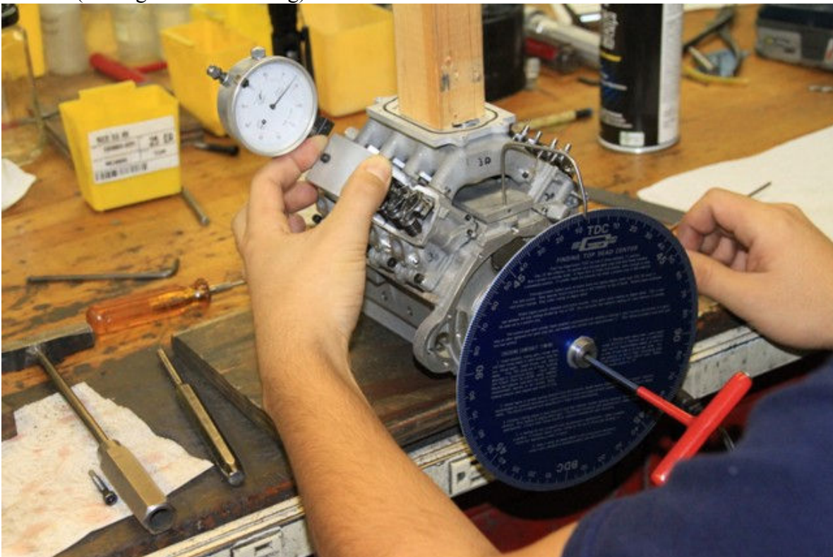
Pic #16 (Setting camshaft timing)
