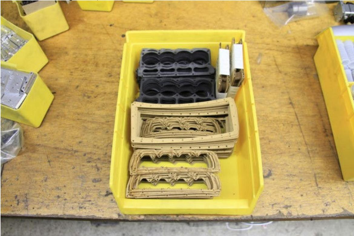
Pic #7 (Laser cut gaskets)
