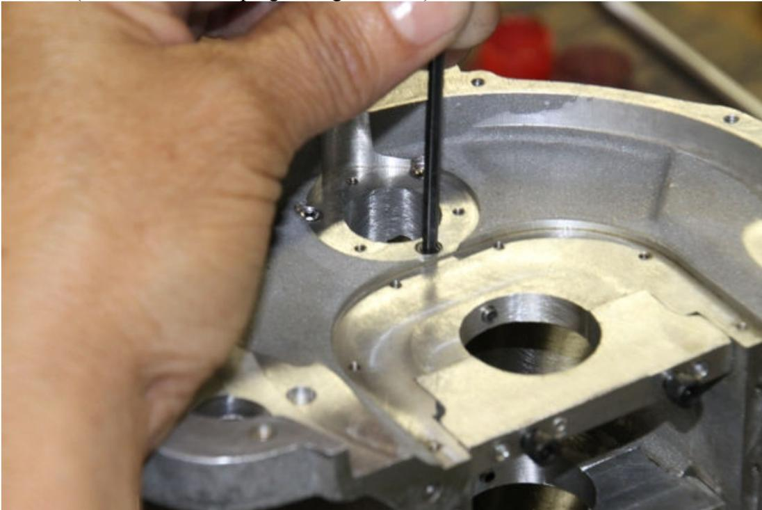
Pic #11 (Oil inlet hole being drilled)
