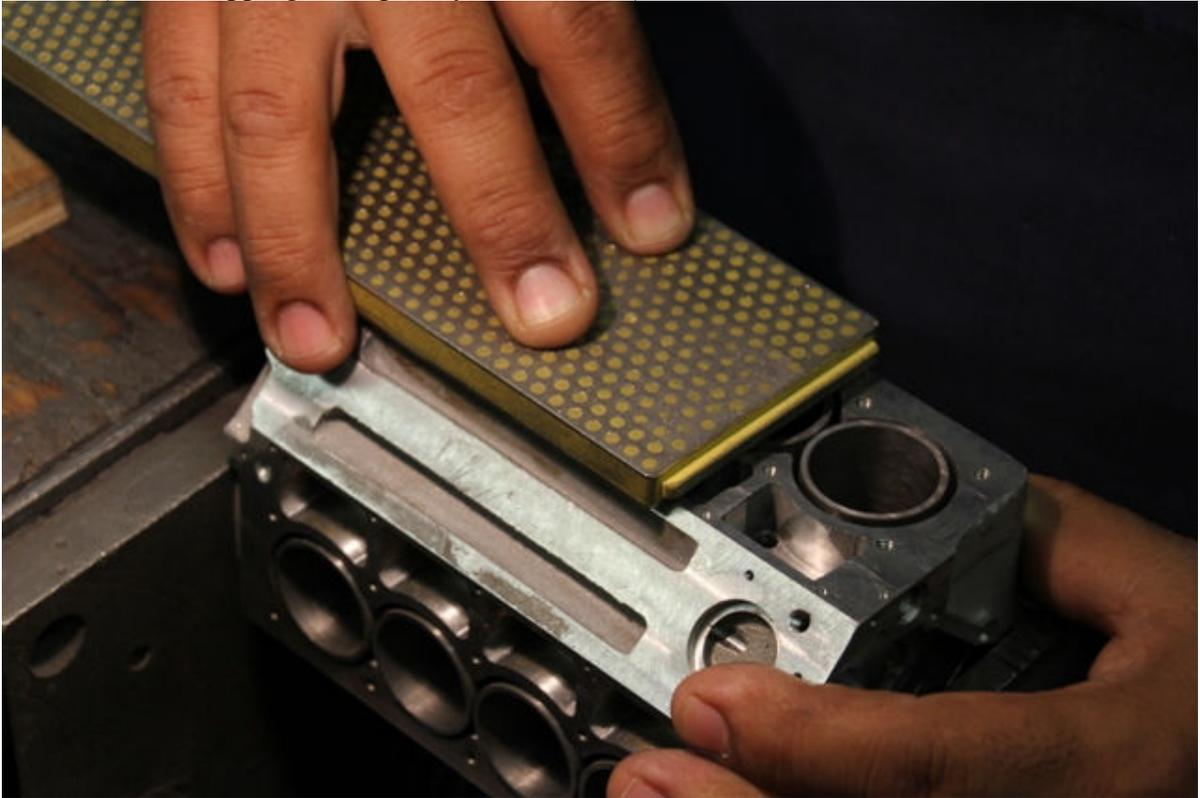
Pic #2 (Fine lapping the top of cylinder liners)
