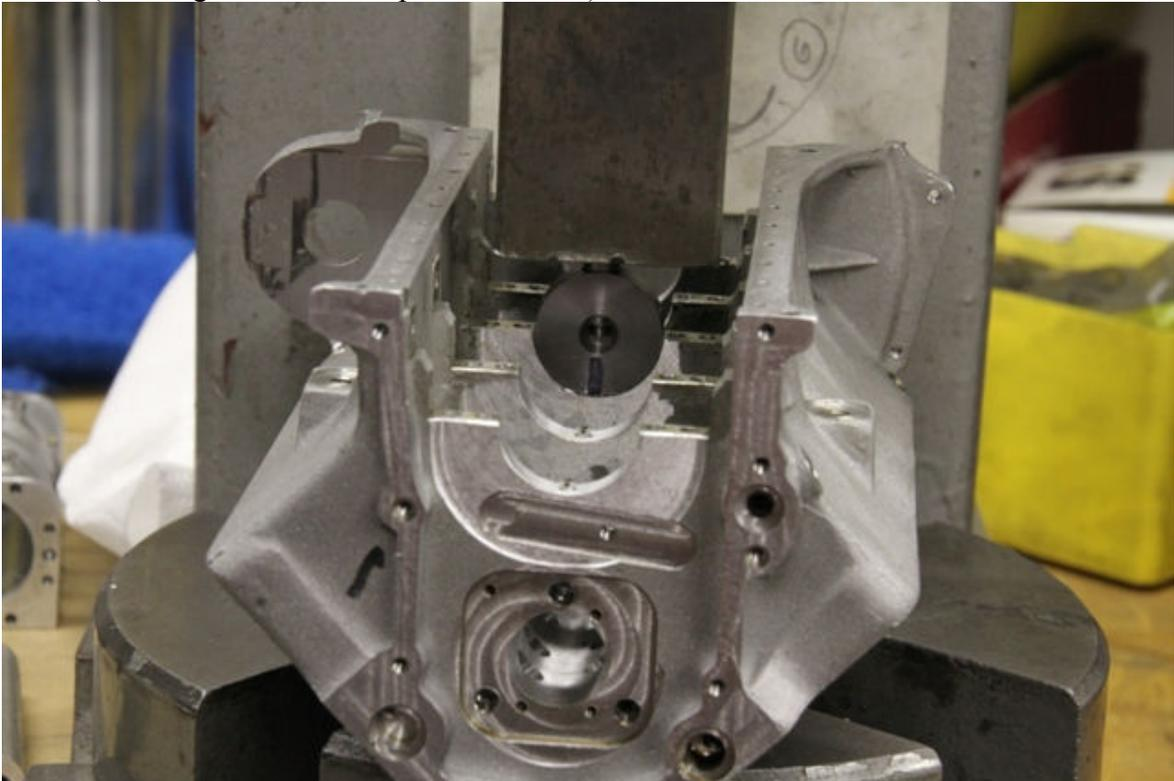
Pic #9 (Brass oil line installed)
