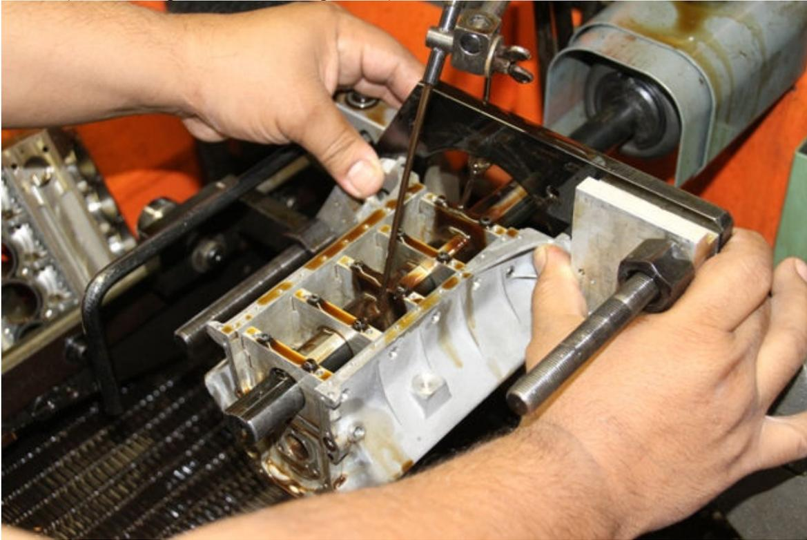
Pic #4 (Line honing camshaft bore)
