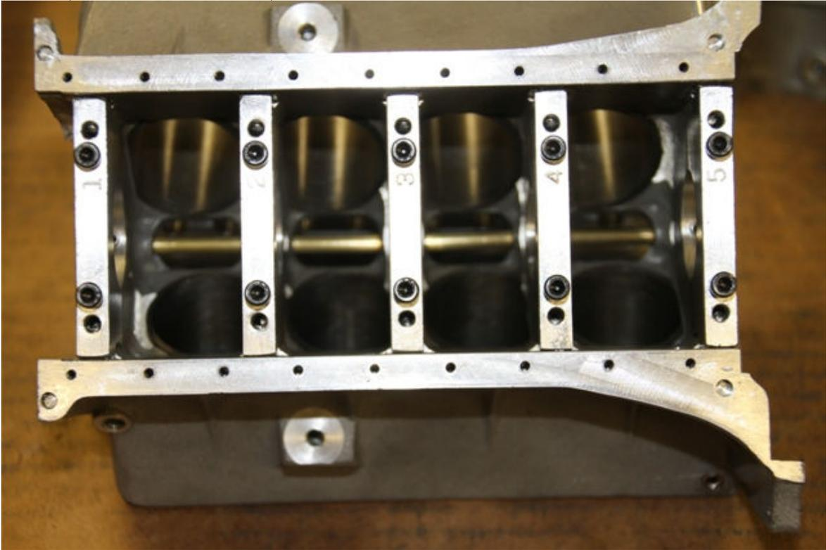
Pic #10 (Stainless steel oil plugs being installed)
