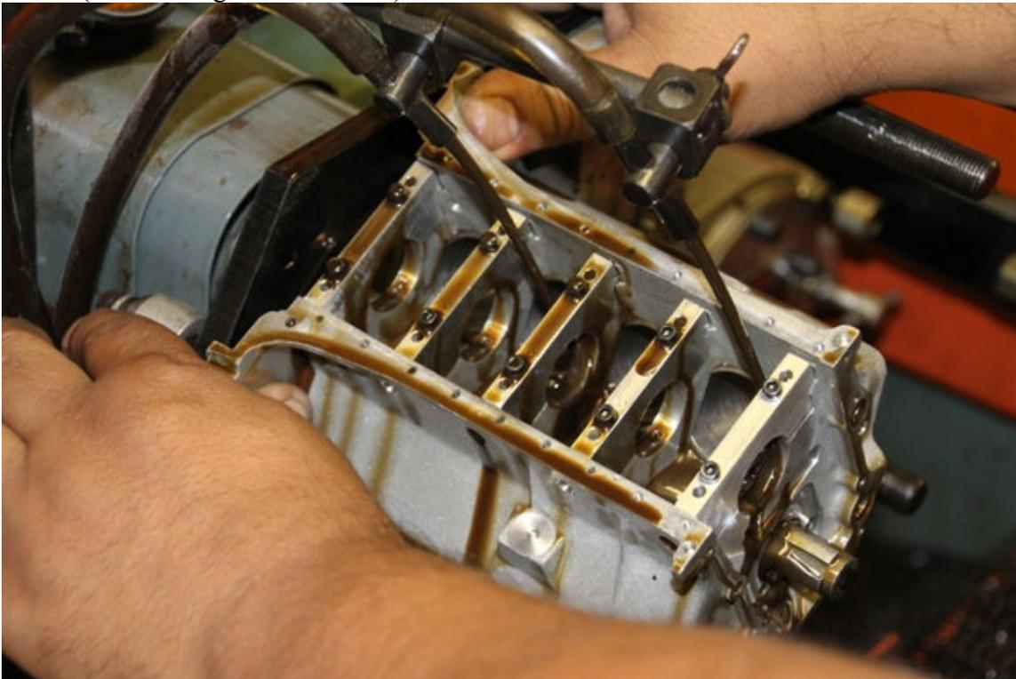
Pic #5 (Check camshaft bore)
