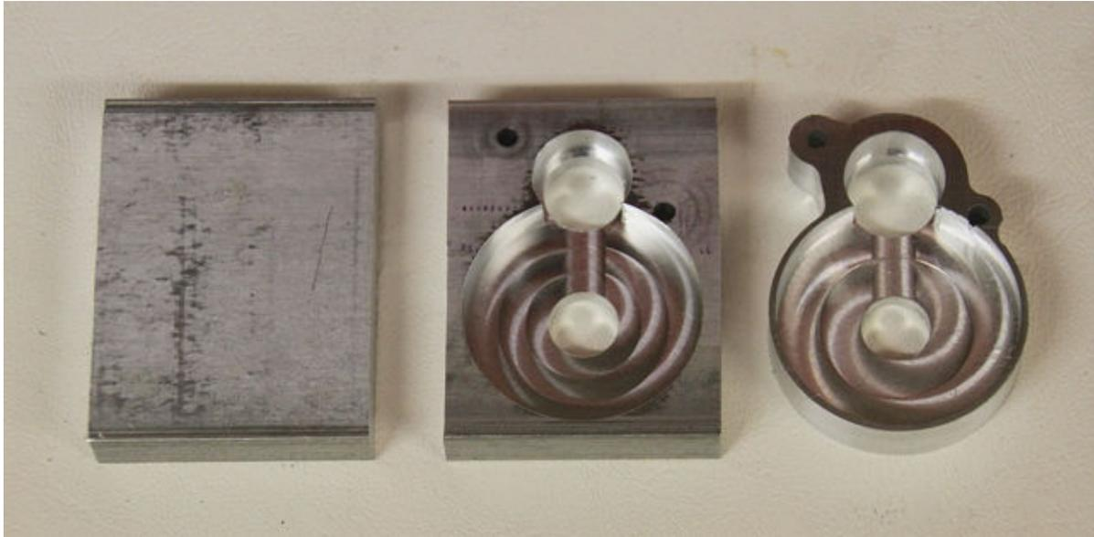
Pic #3 (Completed gear case housings)
