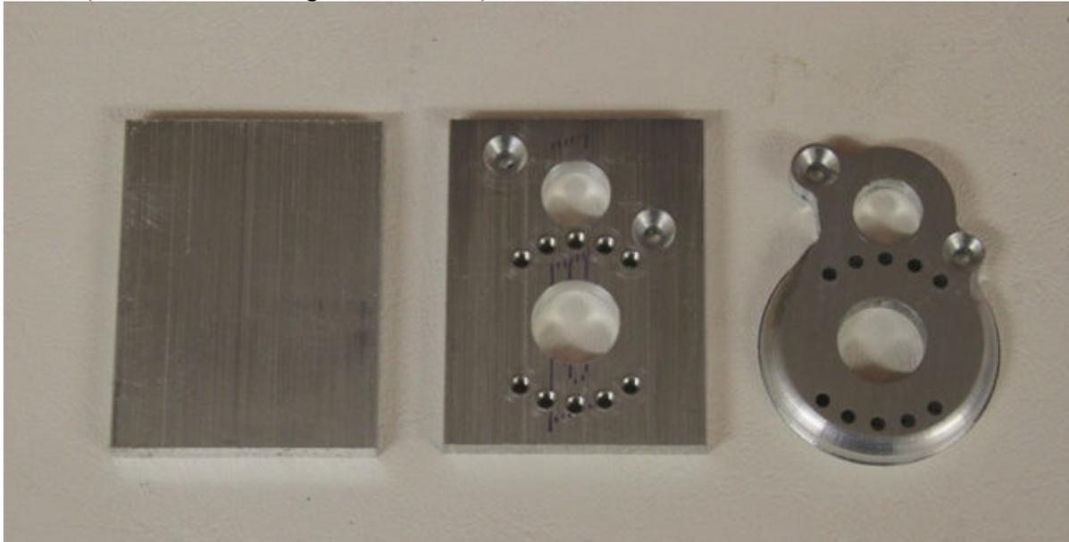
Pic #2 (New starter motor gear case)
