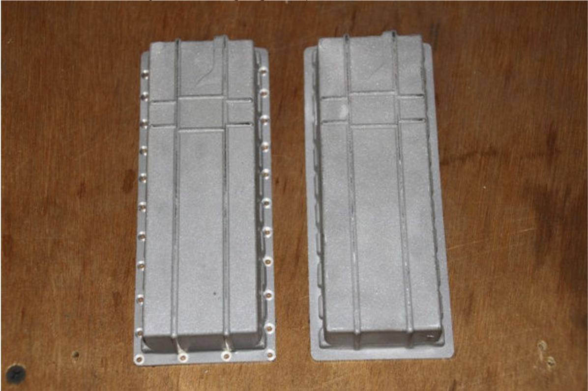
Pic #4 (Finished pans with quick disconnects installed)
