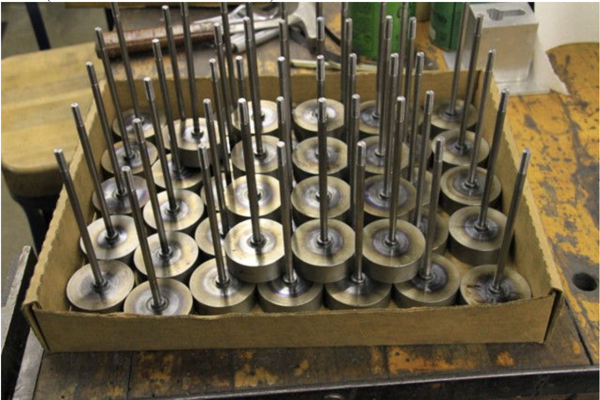
Pic #8 (Welded drive shaft and clutch bell)
