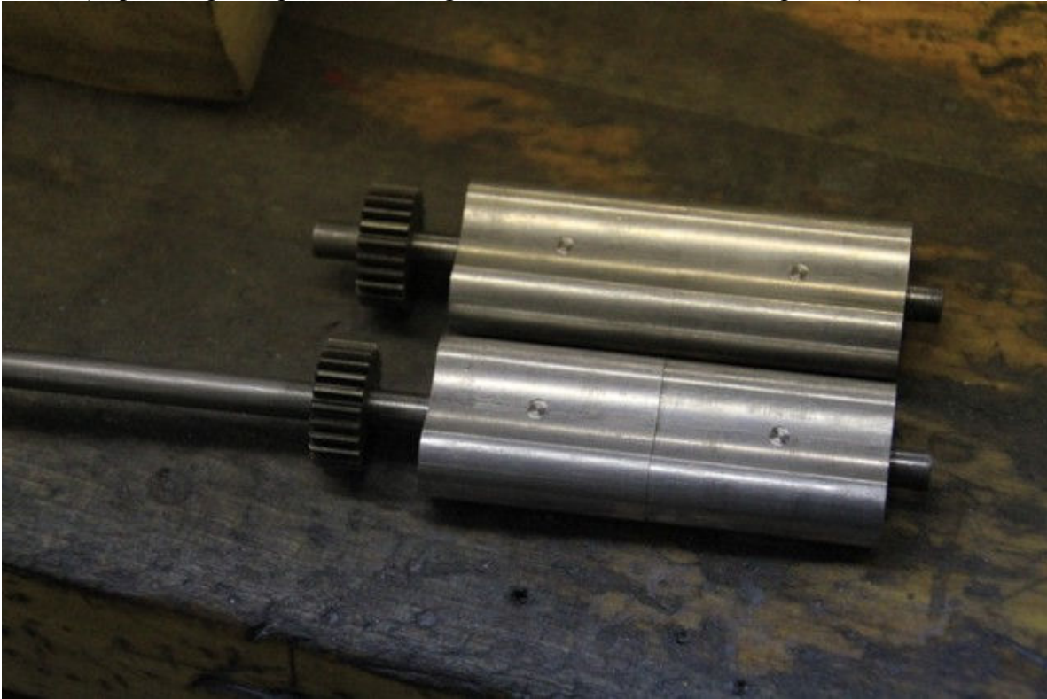
Pic #6 (Completed and matched sets of supercharger impellers)
