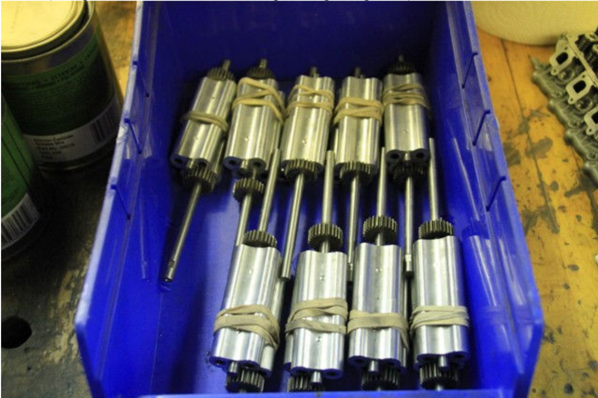
Pic #6 (Completed and matched sets of supercharger impellers)
