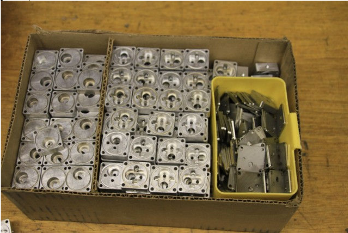
Pic #5 (Lot of front, center gear sections, and thrust plates ready to start the assembly process)
