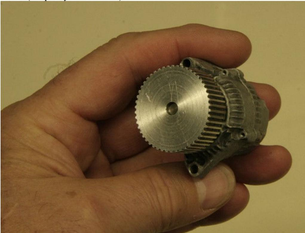
Pic #8 (new pulley on alternator)
