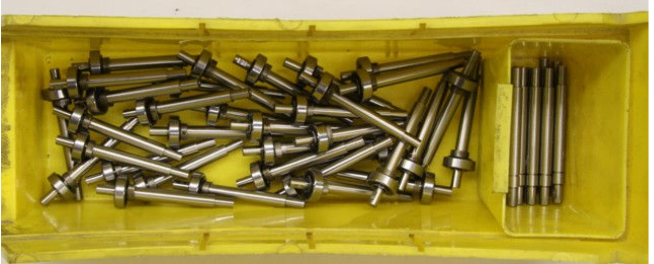
Pic #5 (Completed distributor shafts)
