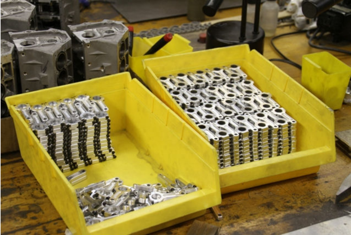
Pic #3 (Connecting rods with bearing installed on right parts tray)
