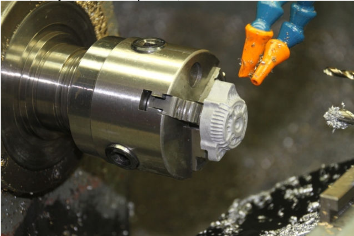
Pic #6 (Holding alternator half in 3 jaw chuck)
