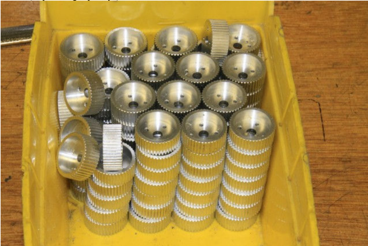
Pic #7 (Finished starter gears)
