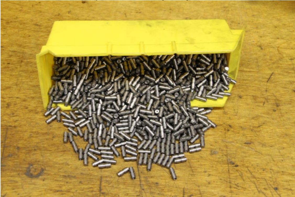
Pic #1 (Finished lifters, ready for heat treat and grinding)
