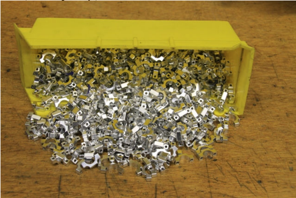
Pic #5 (Connecting rod caps)
